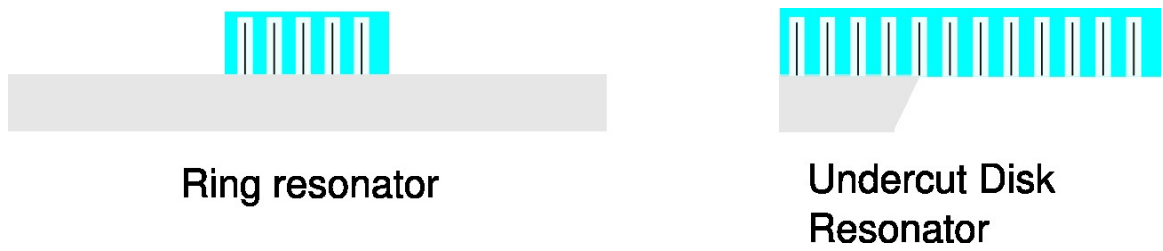
Figure 5.25: The left structure shows the cross-section of a ring resonator built around pillars. The right structure shows the improved confinement afforded by an undercut disk resonator.
