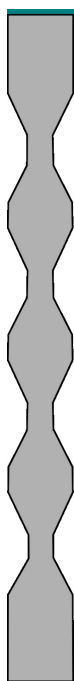
Figure 6.14: Schematic of a vertical stack of dots with equal 'bead' and 'string' diameters made by a modification of both the forward power and the passivation gas flow.
