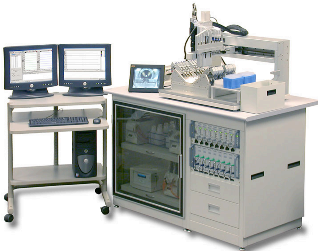
Figure 2.28. The Opus Express system used for most experiments requiring two-electrode voltage clamp electrophysiology.
