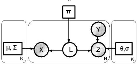
Figure 3.5: The graphical model for the maximum likelihood density estimation for learning from both vision and automatic mechanical supervision. The observed random variables are displayed in shaded circles.
