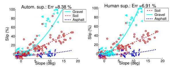
Figure 4.6: The learned slip models and the classification of the test examples when learning with automatic supervision (left) and learning with human supervision (right). The examples are marked according to their predicted terrain class labels (the colors and markers are consistent with Figure 3.3).
