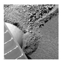
Figure 1.1: The Mars Exploration Rover Opportunity trapped in the Purgatory dune on sol 447. A similar 100% slip condition can lead to mission failure. Image credit: NASA/JPL, Caltech.
