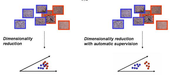
Figure 4.2: Schematic of the main idea: The supervision signals are incorporated in the system so that they affect the dimensionality reduction as well as the classification.
