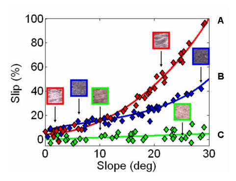
Figure 3.2: A schematic of the main learning setup using automatic supervision: several unknown nonlinear models describe the mechanical behavior corresponding to different terrain types; each training example consists of a vision part (e.g., an image patch of this terrain) and one single point on the curve (marked with a diamond) describing the mechanical behavior.
