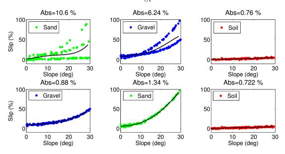
Figure 3.8: The learned nonlinear models for the three classes superimposed on the training data. Learning without supervision (top), learning with automatic mechanical supervision (bottom). The slip models could not be estimated correctly in the unsupervised case because of initial errors in the terrain classification. They are learned correctly after adding the supervision.
