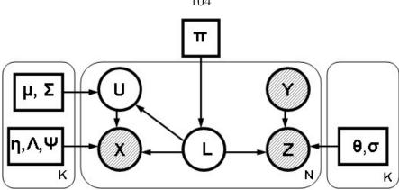
Figure 4.3: Graphical model of the proposed supervised nonlinear dimensionality reduction in which additional ambiguous and noisy measurements are used as supervision. The left part of the graph is essentially unsupervised dimensionality reduction based on MFA [102] with the small but crucial difference that the variables U will be hidden in the proposed algorithm.
