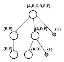
Figure 5.3: Schematic of the proposed variable-length representation. The algorithm has hierarchical structure. Each level applies a more complex classifier. A decision whether to subdivide the recognition task into several groups of non-overlapping classifications is made at each level. The terminal nodes are shaded; these classes do not need to be further trained or classified.
