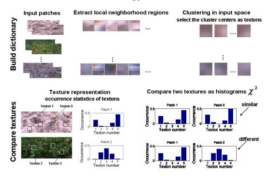
Figure 2.10: Schematic of the terrain classification algorithm [79, 123].
