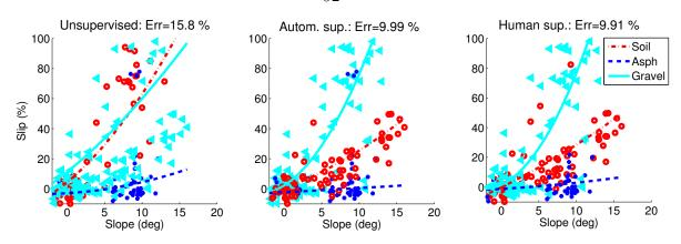
Figure 3.11: Field data test results for one of the runs. The learned nonlinear slip models superimposed on the test data when learning without supervision (i.e., unsupervised) (left), when learning with automatic supervision (middle), and when human labeling is used (right). The test errors for this run are given atop each plot.
