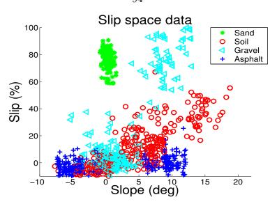
Figure 3.12: Missing data problem extension. Slip measurements plotted as a function of the estimated slope angles retrieved from actual rover traversals. Data for some slope ranges may be unavailable, as is true here for the sand terrain. This may be indicative of the rover not being able to traverse any larger slopes and may be sufficient information to learn the whole slip model. LAGR vehicle
