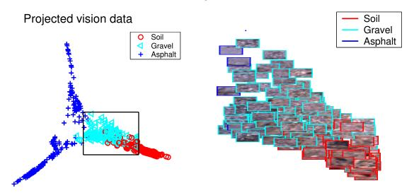
Figure 4.1: Terrain patches and their lower-dimensional projections obtained by the unsupervised dimensionality reduction algorithm Isomap [115]. The original patches corresponding to the projections of the data points in the rectangle are displayed to the right.
