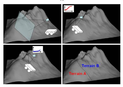
Figure 3.1: An autonomous vehicle uses stereo vision to obtain information about terrain ahead (top left). Measurements about the mechanical vehicle-terrain interaction, or slip, can be collected at different traversed locations by the vehicle's onboard sensors (top right and bottom left). These measurements can be used as supervision to infer that the terrain types are different (bottom right) and to also learn their inherent slip properties for the purposes of future slip prediction.
