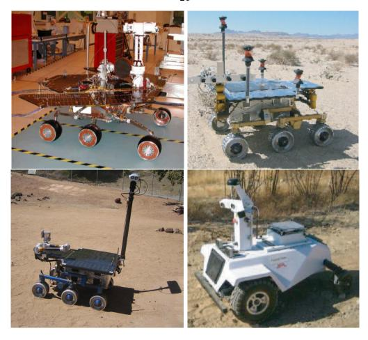
Figure 2.2: Robot platforms. The Mars Exploration Rover Spirit in the JPL Space-craft Assembly Facility (top left). The Rocky8 rover in the Mojave desert (top right). The Pluto rover in the JPL Mars Yard (bottom left). The LAGR robot on off-road terrain (bottom right).
