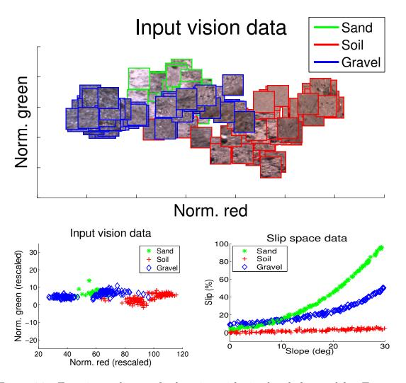
Figure 3.7: Experimental setup for learning with simulated slip models. Top row: Example terrain patches displayed in the initial vision space with ground truth classification (only a subset of the patches is shown). Bottom row: 2D color representation of the terrain patches (left) and the assigned nonlinear slip models (right).
