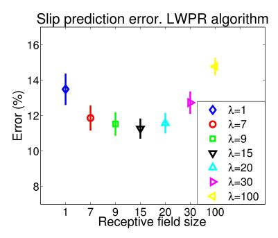
Figure 4.8: Slip prediction with the LWPR algorithm. The best performance here is for  $\lambda=15$ , which is also outperformed by the proposed dimensionality reduction from automatic supervision.
