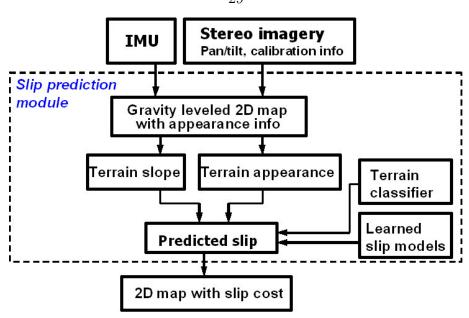
Figure 2.7: Slip prediction algorithm framework.
