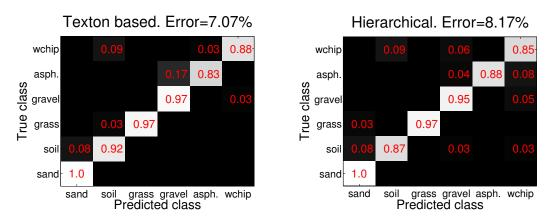
Figure 5.6: Confusion matrices for one of the runs from the results in Figure 5.5. Texton based (left); hierarchical (right). Only the non-zero elements are displayed.
