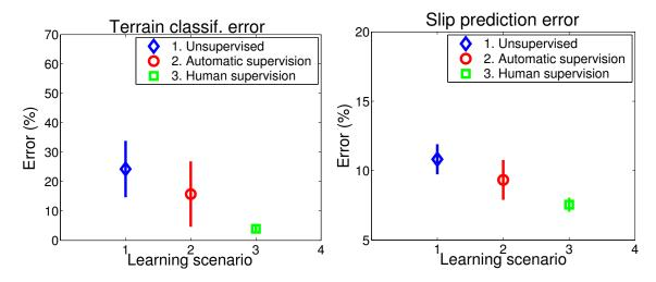
Figure 4.5: Average test results for terrain recognition (left) and slip prediction (right).
