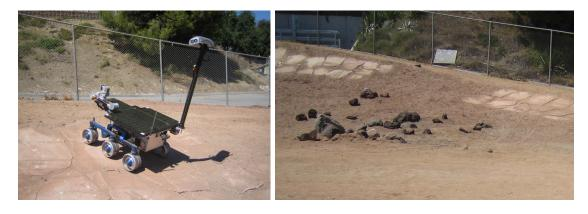
Figure 2.6: The Mars prototype rover Pluto in the JPL Mars Yard (left). An image showing the types of terrains available in this dataset (right).
