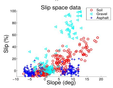
Figure 3.3: Slip measurements plotted as a function of the estimated slope angles retrieved from actual rover traversals. The ground truth terrain types in this figure are provided by human labeling for visualization purposes. The proposed algorithm does not use the ground truth.
