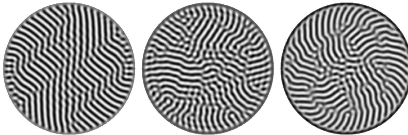
Figure 6.4: Simulation of the Boussinesq equations with \Gamma = 20 , \sigma = 0.93 , \Omega = 17.6 , \epsilon = 0.055 , and an artificially large centrifugal force in order to model the effect of an inaccessibly large \Gamma . Left: zero centrifugal force. Center: centrifugal force is 4 times the physical value. Right: centrifugal force is 10 times the physical value. We used a time resolution of 0.001 for these simulations.
