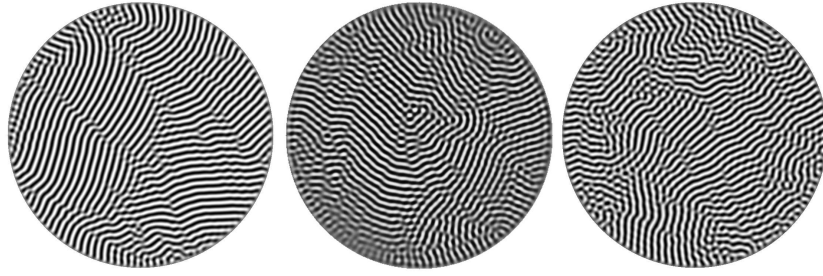
Figure 6.5: Images of domain chaos in Rayleigh-Bénard convection with \Gamma = 36 , \sigma = 0.821 , \epsilon = 0.05 , and \Omega = 16.25 . Left: the temperature profile at the mid-plane from simulation of the Boussinesq equations with no centrifugal force. Center: shadowgraph image from experiment. Right: the temperature profile at the mid-plane from simulation of the Boussinesq equations including centrifugal force.
