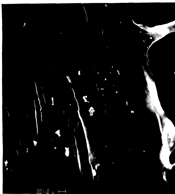
Figure 4.22 SEM of the unoriented PPA:polynorbornene (1:1.2) block copolymer at 20,000 magnification (a); and the oriented block copolymer ( l/l_o=6 ) at 3000 magnification (b).
