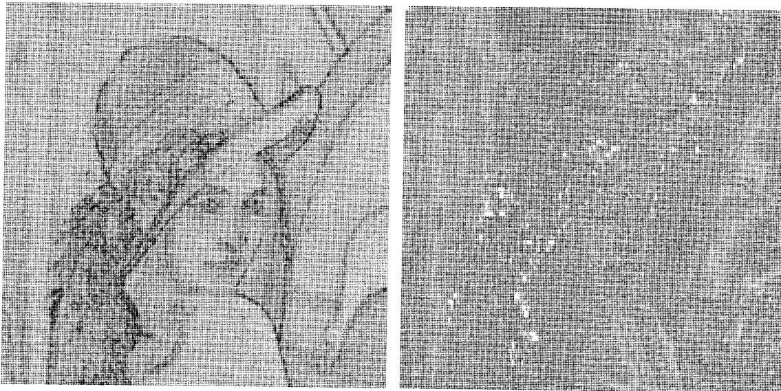
Figure 28: Error images, LAVQ and LBG. Basic LAVQ algorithm (error allowance of 0.0479, 1 \times 8 pixel blocks, and 255 entry code book) and LBG compression ( 4 \times 4 pixel blocks and 256 entry code book) applied to the lenna image. Left image shows error after processing with LBG algorithm; LBG obtained 0.625 bit/pixel compression at a pixel-wise mean squared error of 6.744 \times 10^{-4} . Right image shows error after processing with basic LAVQ algorithm; to obtain a comparable error 6.700 \times 10^{-4} , a rate of 1.33 bits/pixel is needed.
