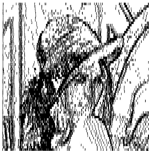
Figure 41: Nonrepeating codeword locations. Nonrepeating codeword locations for the lenna image. Note that the LAVQ algorithm picks out edges and areas of high detail well. Coding parameters were identical to those used in Figure 28.
