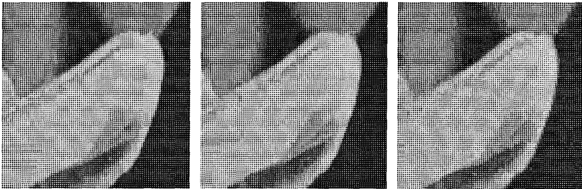
Figure 36: Bit stripping detail. Detail of upper right edge of hat brim from the lenna image using the basic LAVQ algorithm. From left to right: zero, two, and four bits stripped off the new codewords.
