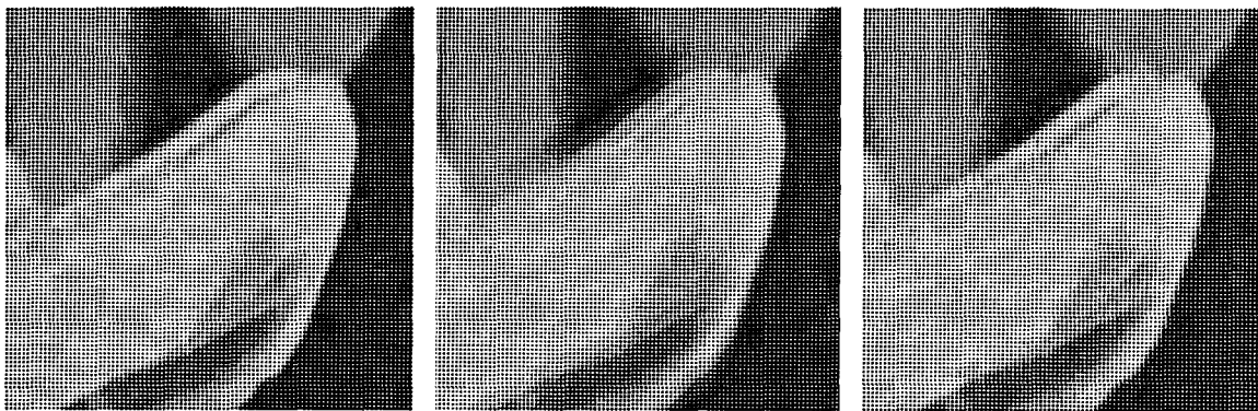
Figure 42: Filtering with block replacement detail. Detail of upper right edge of hat brim from the lenna image. From left to right: basic LAVQ algorithm, filtered image (with attenuation a_0 = 1.0 ), and filtered image with block replacement.
