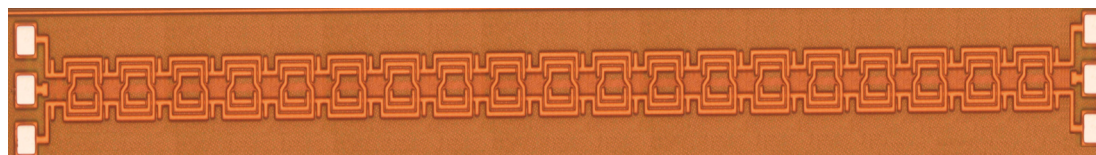
Figure 6.14: Die photo of 19-section VPP-based LC delay line
