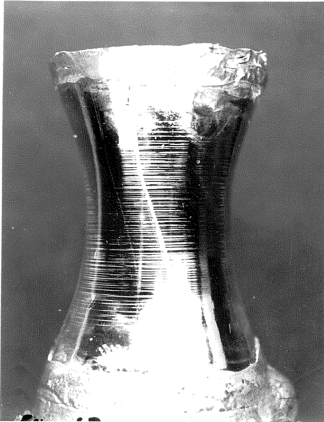
Fig. 29 Coarse Slip Bands Parallel to the Basal Planes of Zinc. 2.25 X
