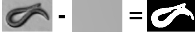
Figure 5.6: Because the background of the petri dish remains largely static, accurate segmentation of the observed data images I_k is achieved using background subtraction.
