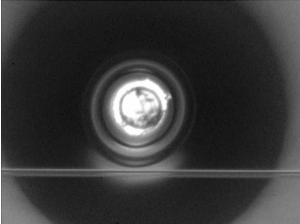
Figure 3-5: A top view optical micrograph of the tunable microtoroid resonator during testing. The aluminum ohmic contact and the fiber taper waveguide can clearly be seen.
