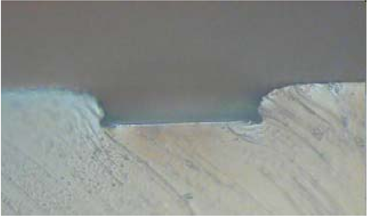
Figure 5-2: Cross-section of the PDMS mold, note the outline of the pillar as well as the toroid ring.
