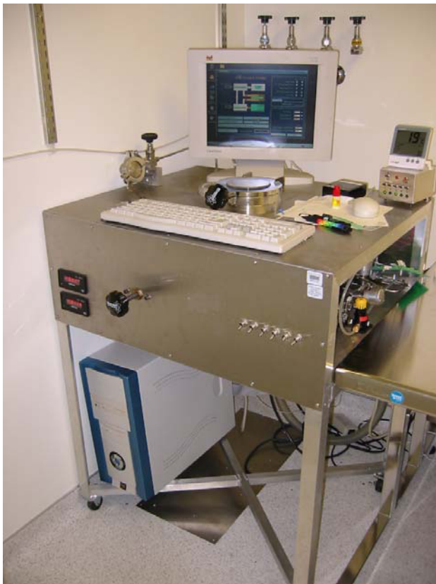
Figure 2-3: A schematic diagram of the xenon difluoride etch system (top). A picture of the actual system in the Vahala lab cleanroom (bottom).
