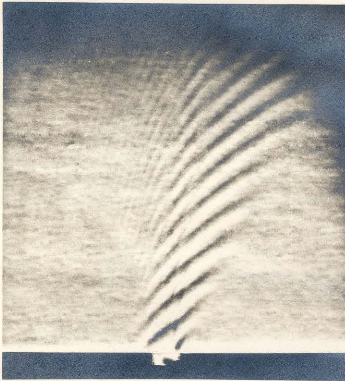
Fig. 1. Sound radiation due to high speed flow over a cavity.
