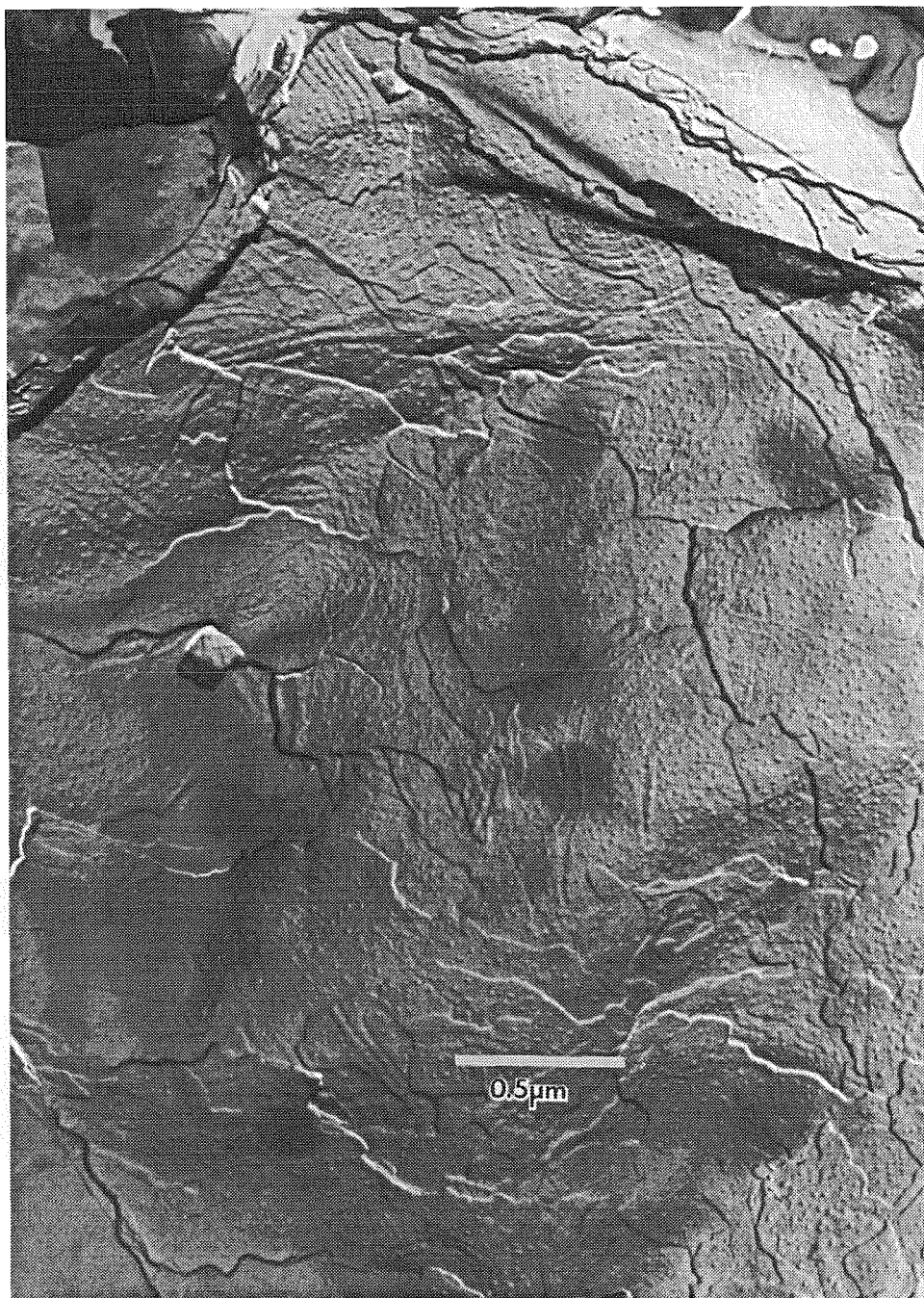
Figure 2.8. Transmission electron micrograph showing freeze-etch prepared DSPC multilamellar vesicles. Magnification is 18,500x; size bar is indicated.
