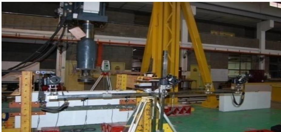
Figure 3: DSLR cameras fixed on steel bar
