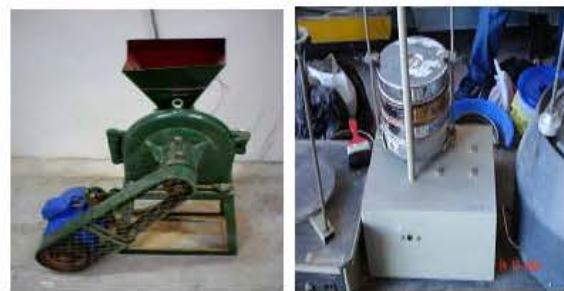
Fig. 2: Grind machine (left) Automatic sieve shaker (right)
