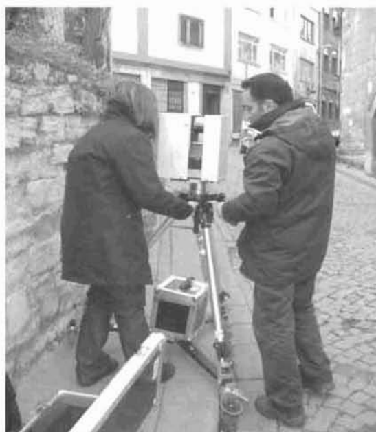
Figure 2 The Optec laser scanning system
