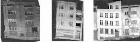
Figure 5 Geometric problems from direct geo-referencing of point clouds (from left to right: swinging façade, misfit at block corner, and deformation of a façade)
