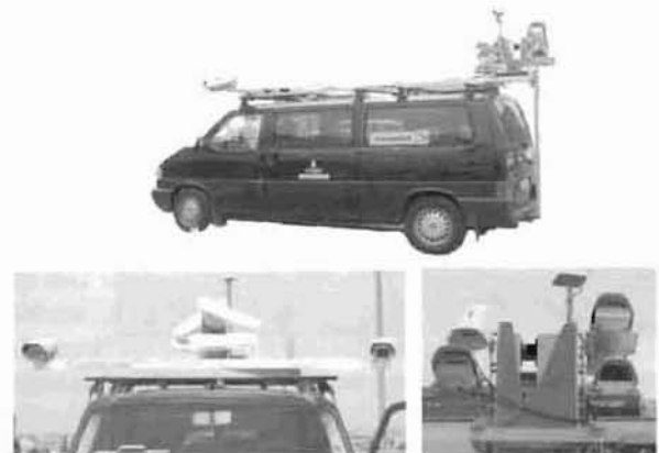
Figure 4 Sensor configuration on the mobile mapping van of VISIMIND AB
