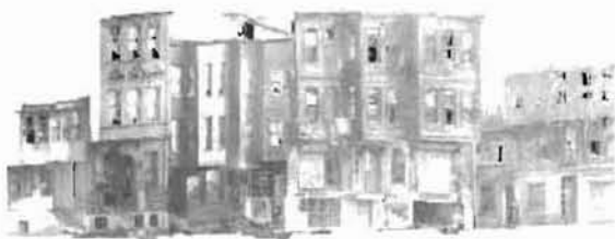
Figure 3 Example of a coloured point cloud of building facades at the Historic Peninsula
