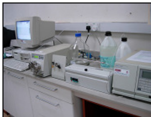
Figure 1.0: HPLC equipment - Isocratic solvent system
