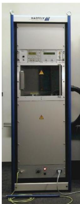
**Figure 3.12** Combination Impulse Waveshapes Generator, HAEFELY PSURGE30
