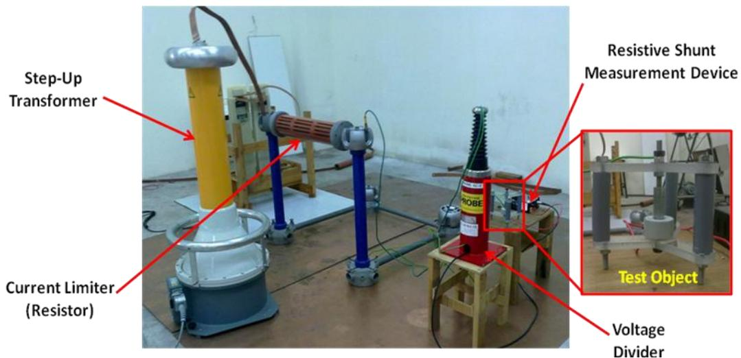
**Figure 3.8** Experimental Setup of Total Leakage Current Measurement
