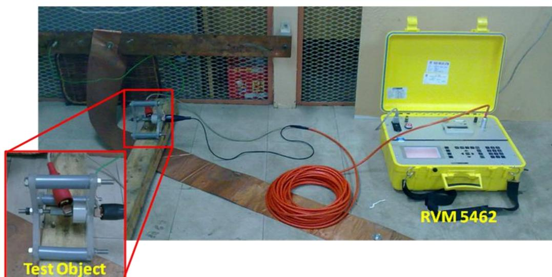
**Figure 3.6** Experimental Setup of RV Measurements
