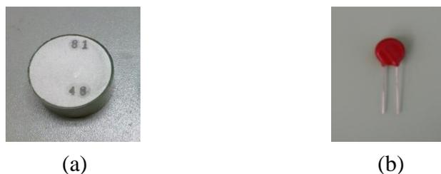
**Figure 3.4** (a) Block-type, and (b) Radial Leaded-type Varistors
