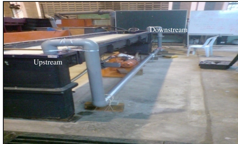
Figure 3.2: The piping system for water re-circulation in the flume
