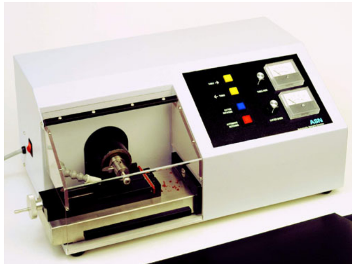
Figure 3.5: The Automatic Notched Machine used to notch the specimens for Izod impact test.
