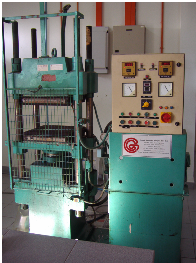
Figure 3.4: The hot press machine for compression moulding samples for flexural, Izod impact and tensile tests.
