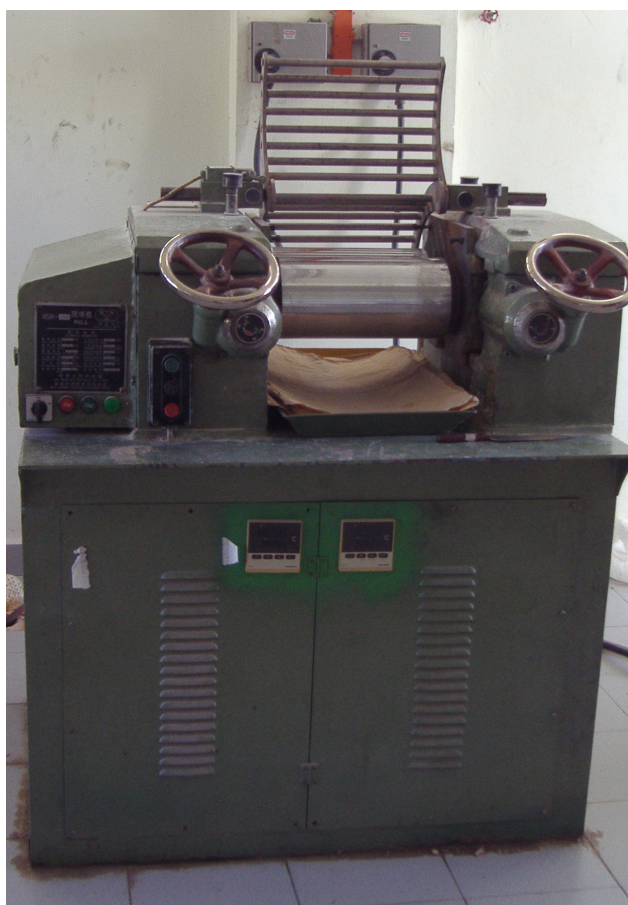
Figure 3.1: The two milling machine used in melting the PVC dry blends.
