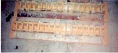
Figure 3.34: Moulds of Mortar Cube
