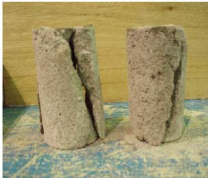
Figure 4.82: Failure Mode of XLPE Modified Mortar Compared to Ordinary Mortar
