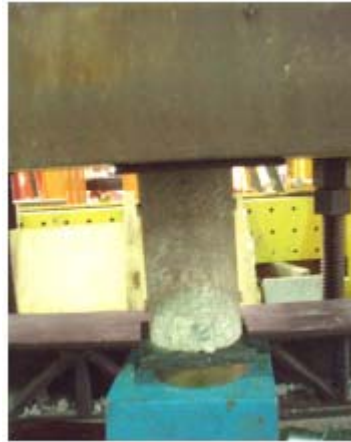
Figure 3.47: Mortar Cylinder with Decmec Points Ready to be Tested
