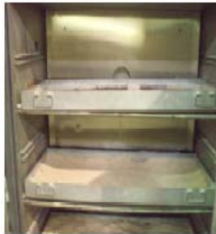
Figure 3.24: Sand Dried in Oven
