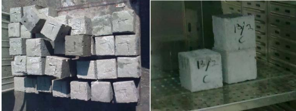
Figure 4.94: Concrete in Room Temperature (left) and Concrete in High Temperature (right)
