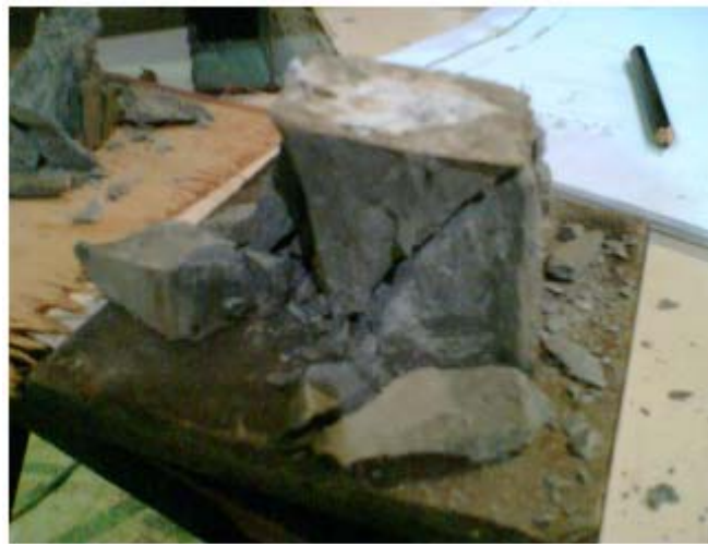
Figure 4.13: Obvious Failure Plane of Control Cube
