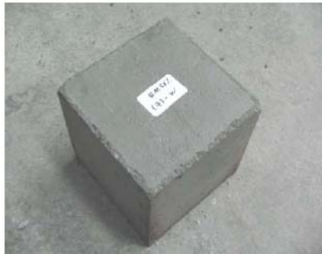
Figure 4.27: The Appearance of 50% EM-AS Concrete Cube
