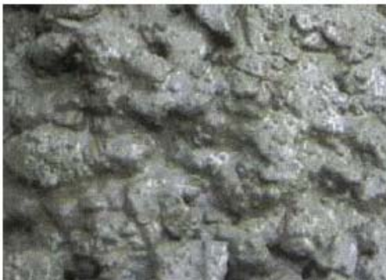
Figure 4.4: Physical Appearance of Concrete with EM-5%
