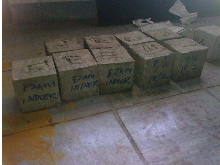
Figure 3.42: Cubes Exposed to the Indoor Environment in the Concrete and Structure Lab, UTM
