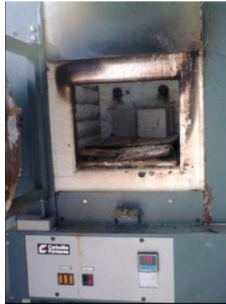
Figure 3.51: Furnace that Can Achieve 2000 °C
