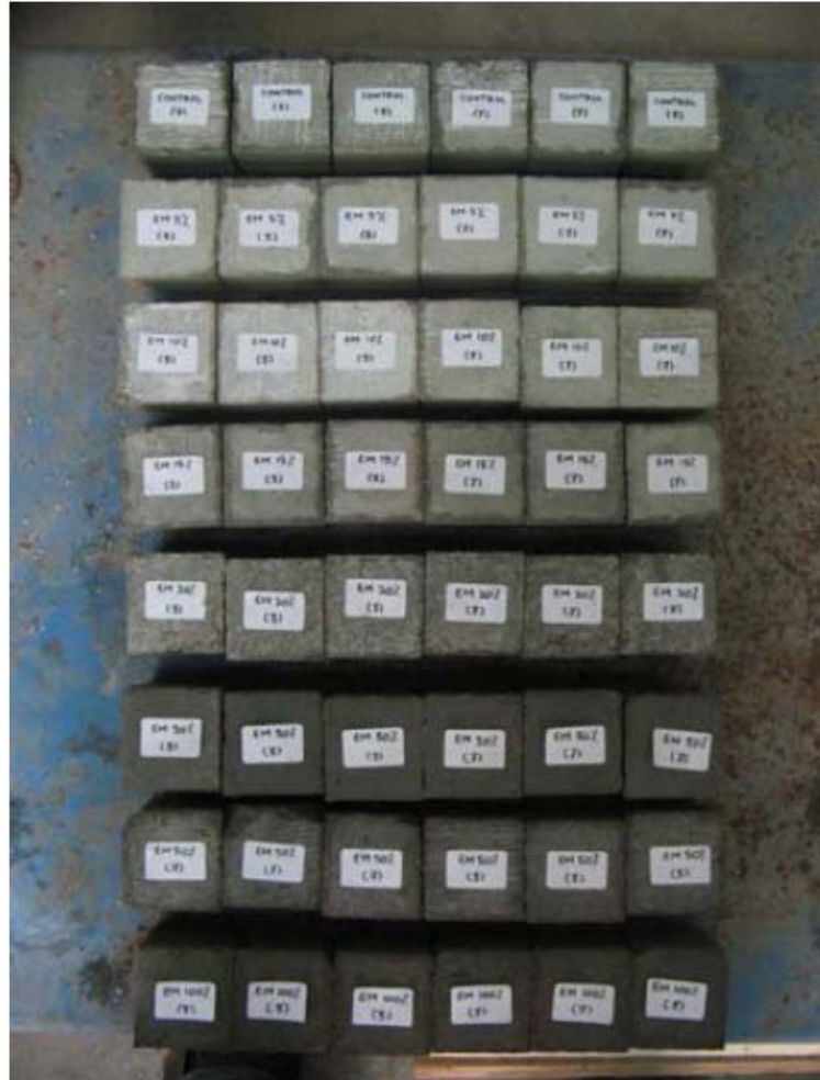
Figure 4.35: Physical Appearance of Mortar Cube Added with Different Proportion of EM-AS.
