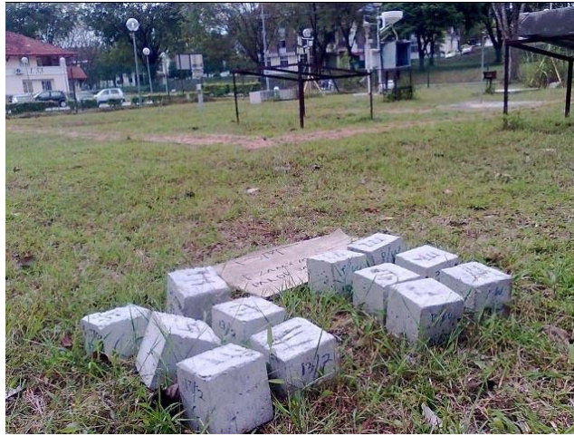
Figure 3.41: Cubes Exposed to the Outdoor Environment in an Open Area Near Arked Cengal, UTM
