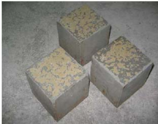
Figure 4.28: The Appearance of 100% EM-AS Concrete Cube
