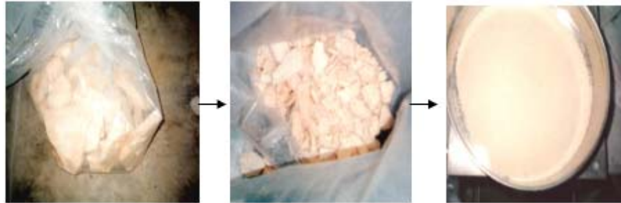
Figure 3.27: Size Reduction of Elastomer-Based Adhesive Waste
