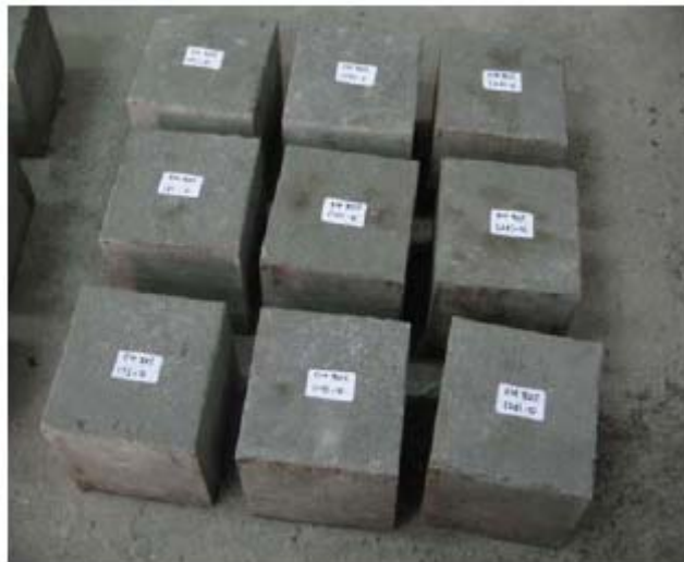
Figure 4.26: The Appearance of 30% EM-AS Concrete Cube
