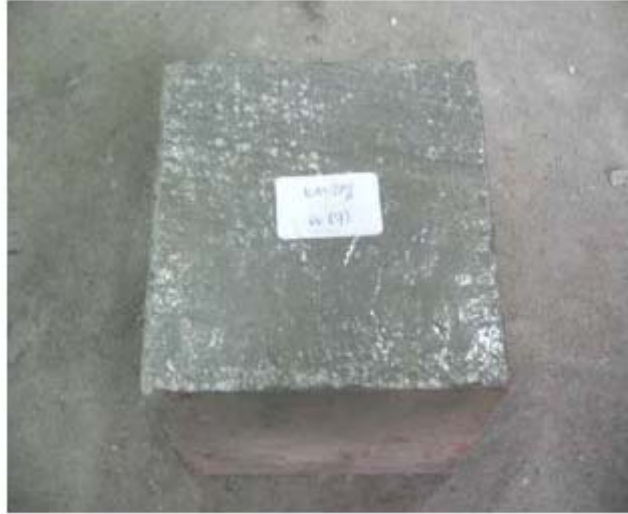
Figure 4.25: The Appearance of 20% EM-AS Concrete Cube
