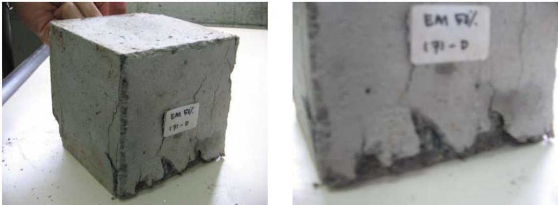
Figure 4.32: Spalling Happened at the Edge of the Concrete Cube before Testing.
