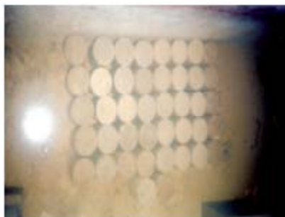
Figure 3.45: Specimens in Wet Curing Condition
