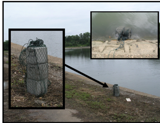
Figure 3.13: Cubes in Net Immersed into Wastewater
