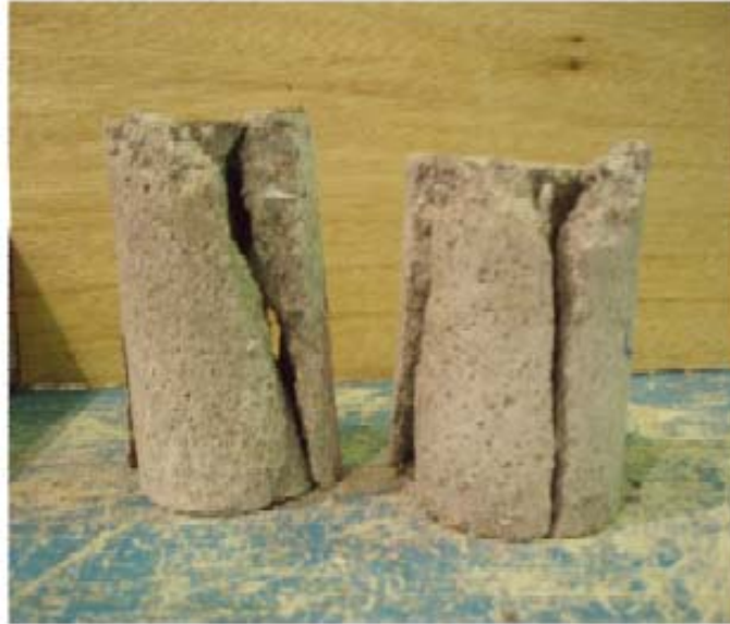
Figure 4.81: Failure Mode of Elastomer Modified Mortar Compared to Ordinary Mortar
