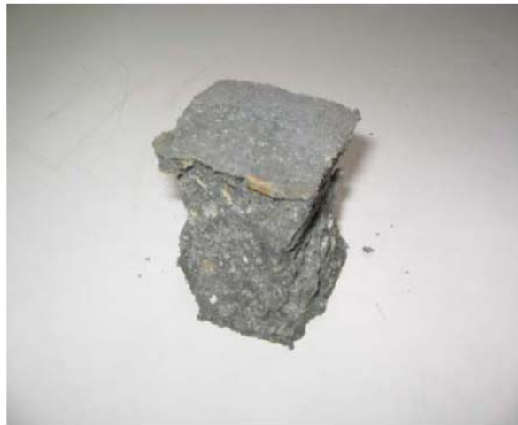
Figure 4.34: Failure Pattern for Mortar Cube
