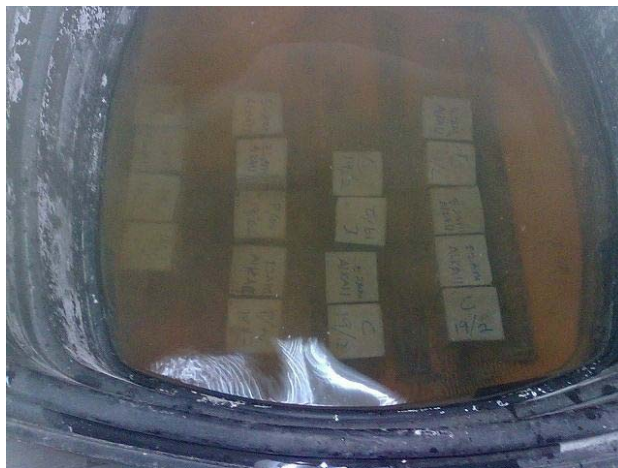
Figure 3.39: Control Cubes and Cubes with Plastic Wastes in the Acidic Solution
