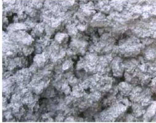
Figure 4.5: Physical Appearance of Concrete with EM-30%
