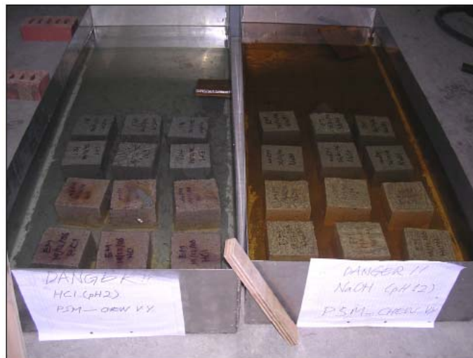
Figure 3.9: Samples in the Acidic Liquid (left) and Alkaline Liquid (right)
