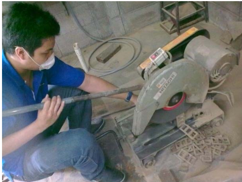
Figure 3.33: An example on How the Fine Particles of Plastic Waste is Collected
