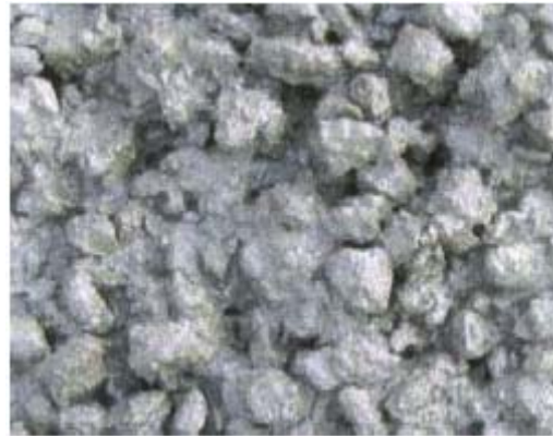
Figure 4.6: Physical Appearance of Concrete with EM-100%
