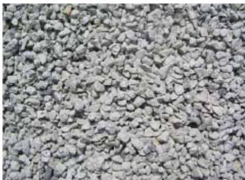
Figure 3.2: Course Aggregate with Maximum Size 10mm.
