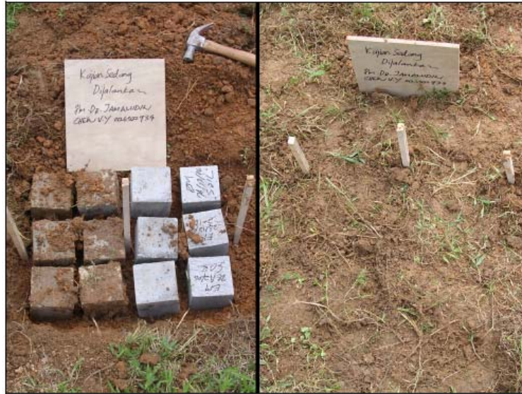
Figure 3.12: Soil Condition; Cubes Being Buried (left) and Cubes Fully Buried under the Clayey Soil (right)
