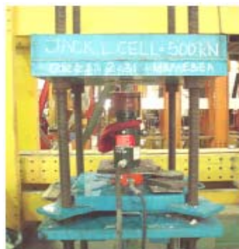
Figure 3.43: Jack Load Cell Used in Compression Test
