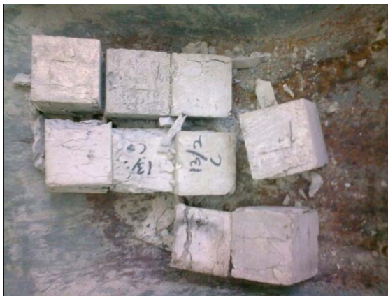
Figure 3.52: Satisfactory Failures for Compression Test
