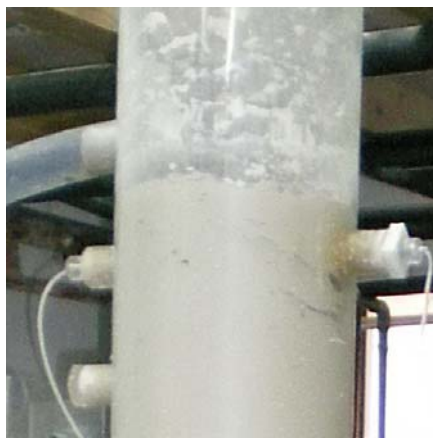
Figure 4.7 Cracks formed at the surface of silt (kaolin)
