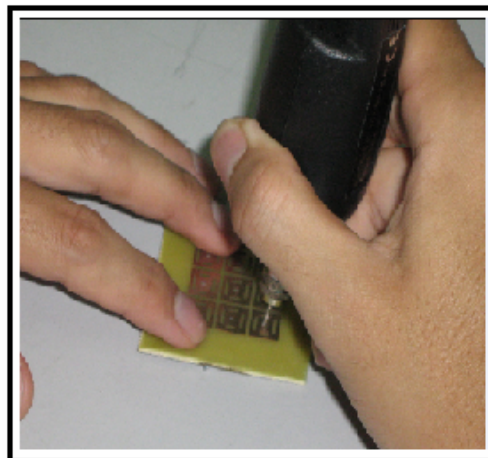
Figure 3.15: Drilling hole at EBG structure
