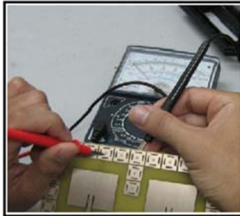
Figure 3.18: Checking the connection of vias to the ground plane.
