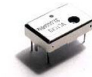
Figure-(6.11) low profile TCXO-514 frequency range 1.2 to 100MHz
