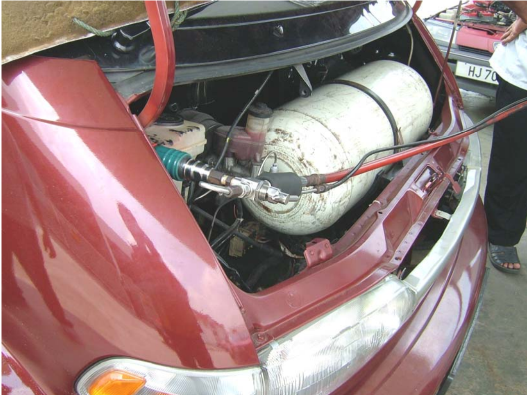
Figure 6.11: Charging of the gaseous fuel into the tank using the filling valve
