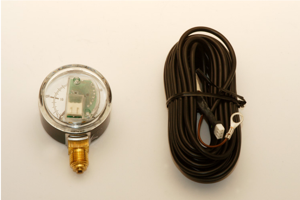
Figure 6.18: Pressure gauge completed with electronic pick-up for level indicator
