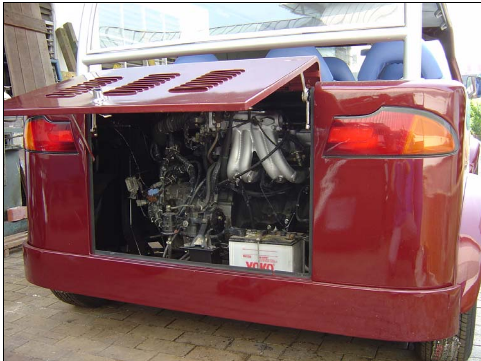
Figure G4: The engine location in tramcar .
