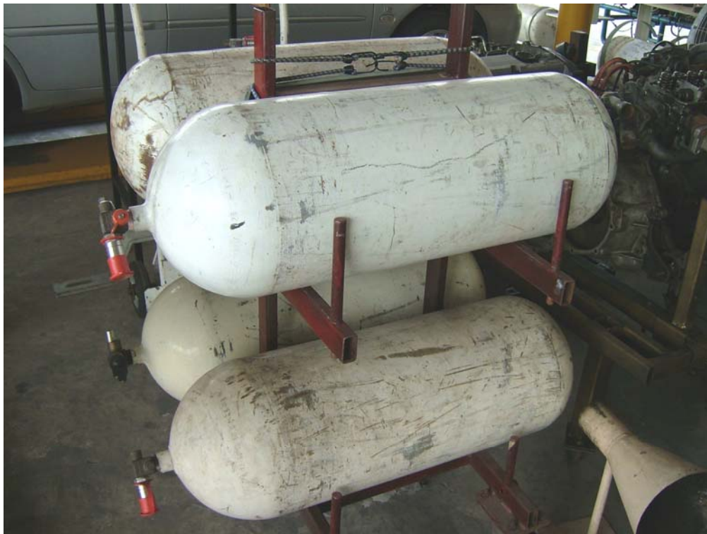
Figure 6.8: CNG steel tanks
