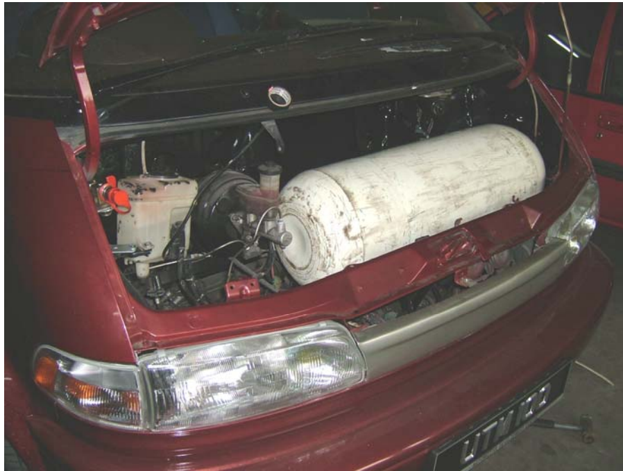
Figure 6.9: Location of CNG tank in the front compartment the Tramcar
