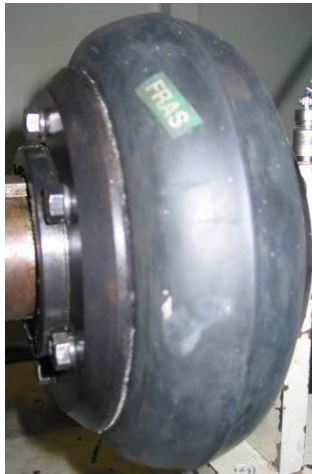
Figure 6.5 Rubber coupling (direct coupling)
