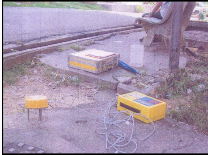
Figure 4.16: Vibration monitoring works in progress.
