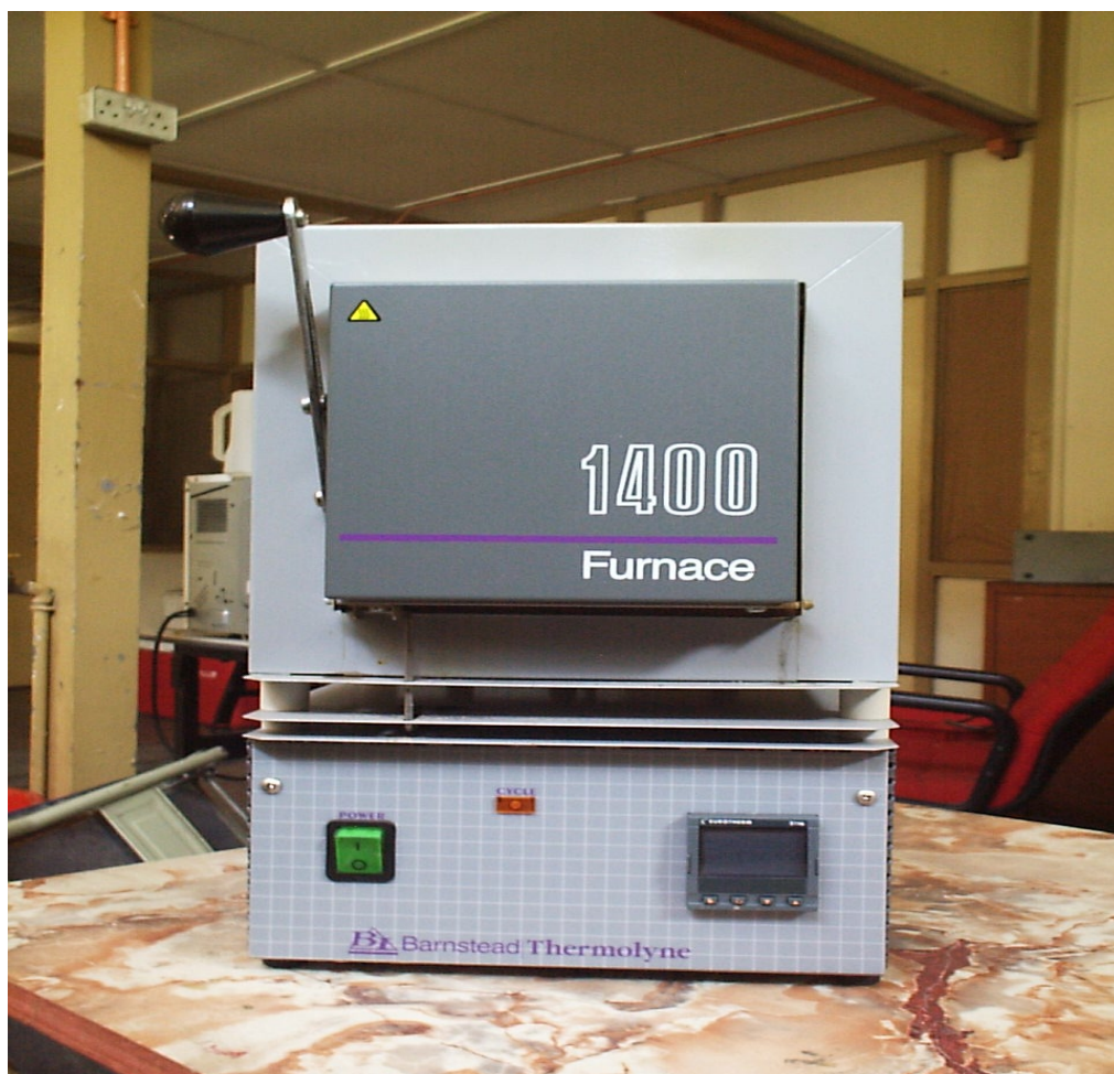
Figure 5.5: Furnace used for the determination of phosphorus content experiment
