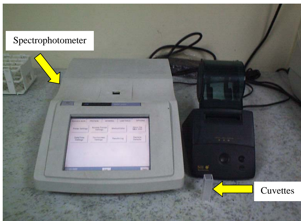
Figure 5.4: Spectrophotometer for determination of DOBI value
