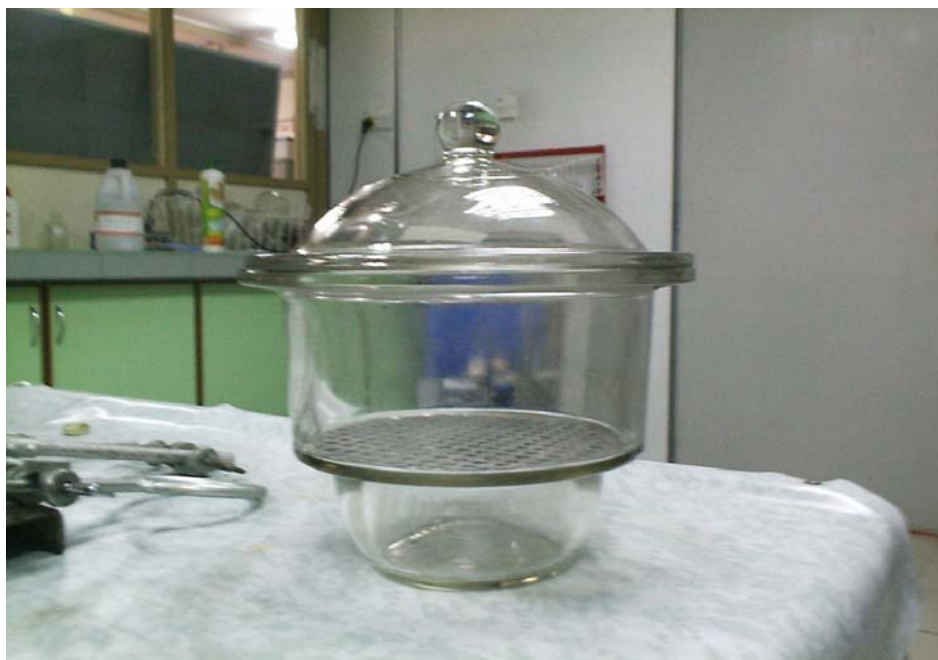
Figure 5.6: Desiccator for moisture content experiment
