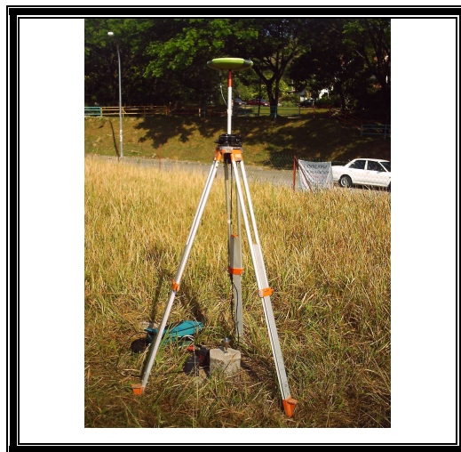
Figure 4.28: Single frequency GPS receiver at W0474 station
