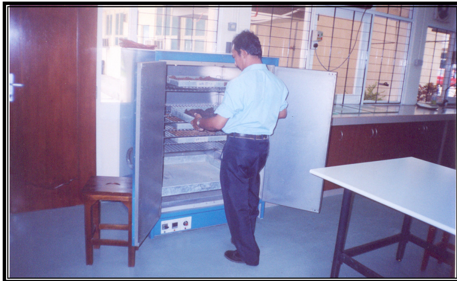
Figure 4.8: Putting the tray into the oven to dry the soil
