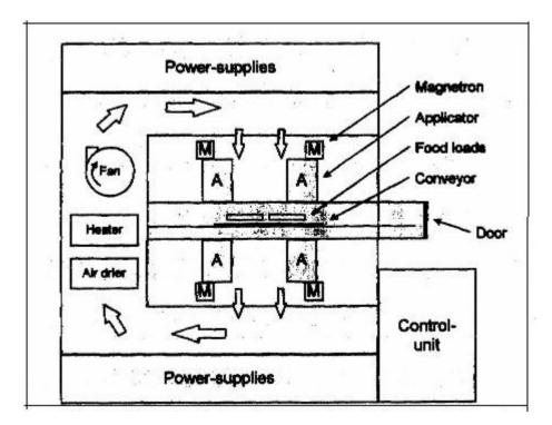
Fig. 5. Schematic illustration of microwave-assisted air dehydration equipment
