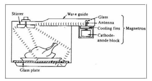
Fig. 2. Microwave oven drying unit
