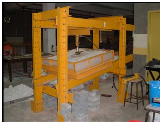
Figure 3.18 Push in test on sloping section
