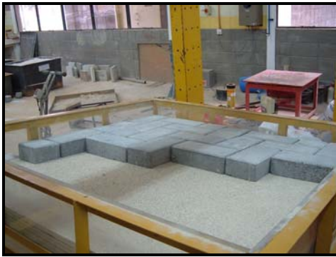
Figure 3.14 Installation of CBP
