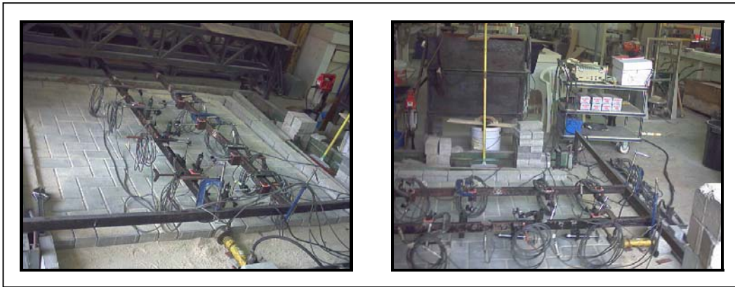
Figure 3.9 Horizontal force test installation
