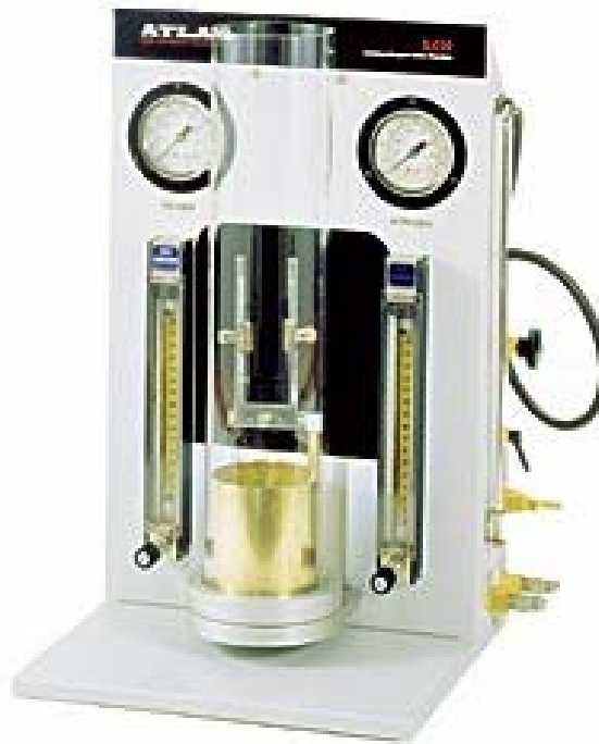
Figure 3.8 : Typical equipment layout for oxygen index test
