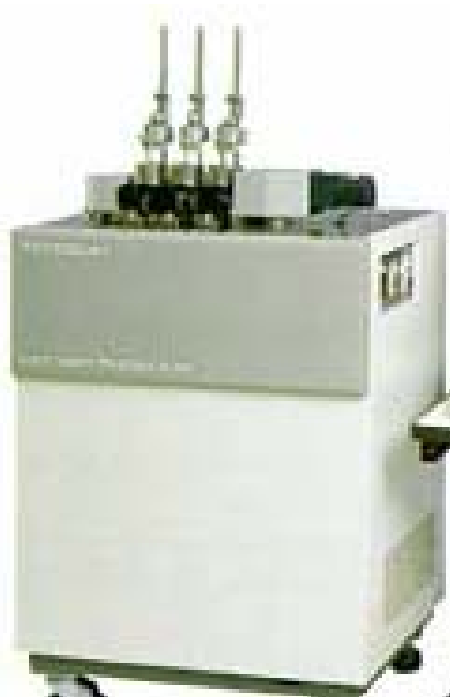
Figure 3.9 : Heat distortion tester S-3 machine
