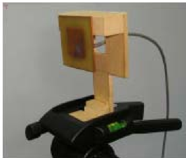
PHOTO F MICROSTRIP PATCH MOUNTED ON TRIPOD FOR POLAR PATTERN MEASUREMENT
