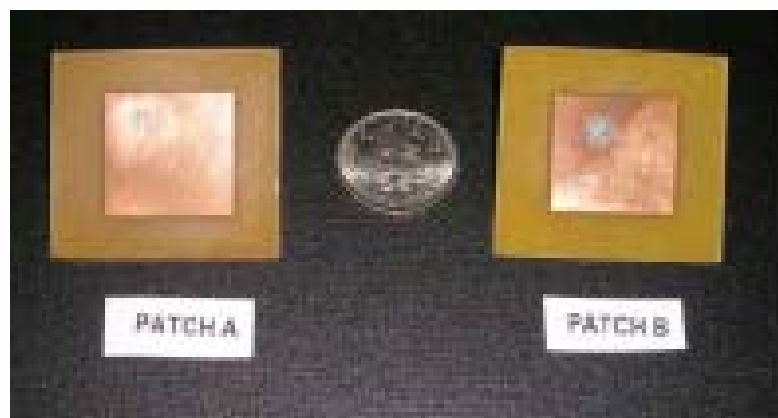
PHOTO B THE CORRECTED DESIGN ANTENNAS
