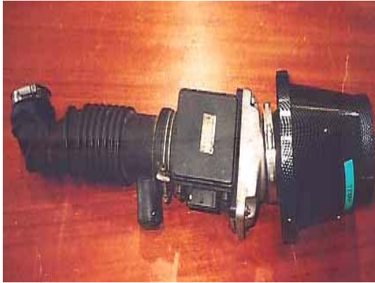
Fig. 3.8: Air filter and flexible hose with mass flow sensor.
