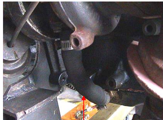
Fig. 3.11: Lube oil drain hose from turbo bearing housing to oil sump.
