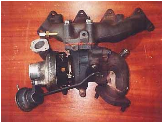
Fig. 3.4: TD05H-16G turbocharger unit with internal waste gate, turbo manifold and turbine discharge pipe.
