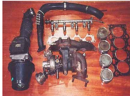
Fig. 3.5: Turbocharger kit complete with metal cylinder head and exhaust gasket.
