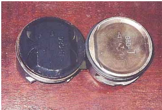
Fig. 3.10: Stock high-compression piston (left) and new low-compression turbo piston (right).
