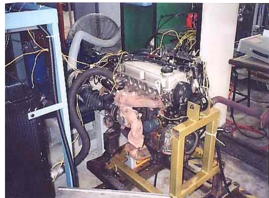
Fig. 3.13: Engine coupled to dynamometer on test bed complete with instrumentations.
