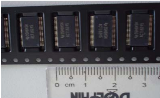
Fig. 4: IC chips in the conveyor
