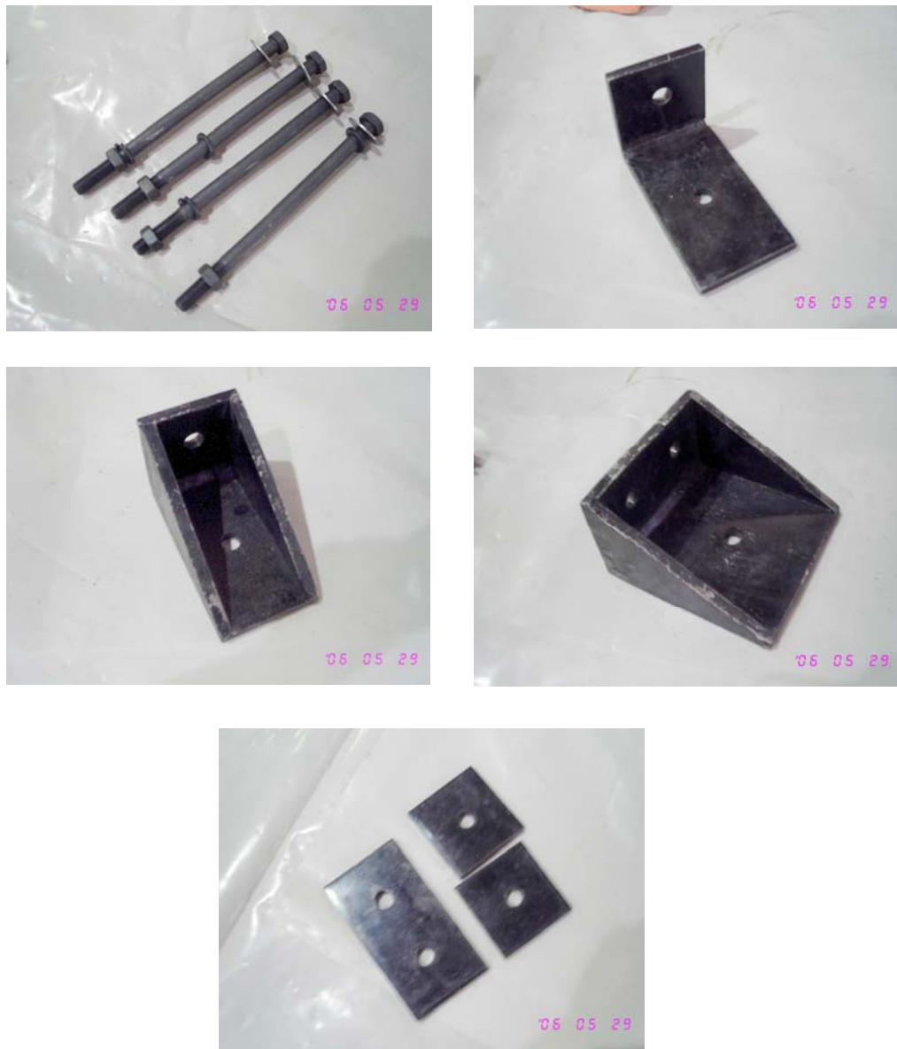
Figure 12 Steel connectors to join the precast beam and column: bolts with nuts, angle cleat, stiffened angle cleats, plates (from left, clockwise)
