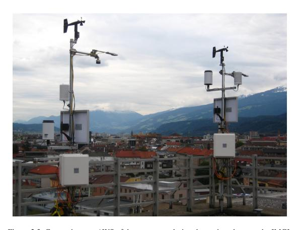
Figure 2.3: Comparing two AWS of the same type during the testing phase on the IMGI.
