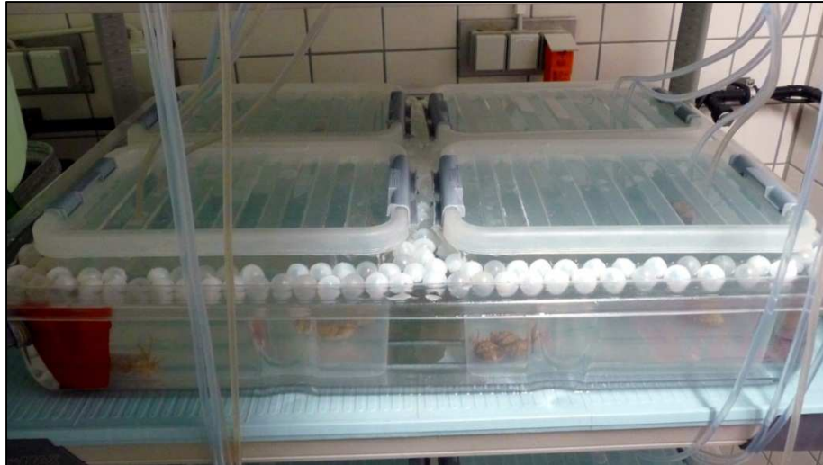
Fig. 2.3: Four incubation boxes in an overflow basin. The boxes are covered with lids. The cuttlefish are visible on the bottom of the front boxes (brown). Each box was supplied by two water tubes from the header tank to increase the water throughput. The water surface of the overflow basin was covered with buoyant plastic balls (H+H incubation).
