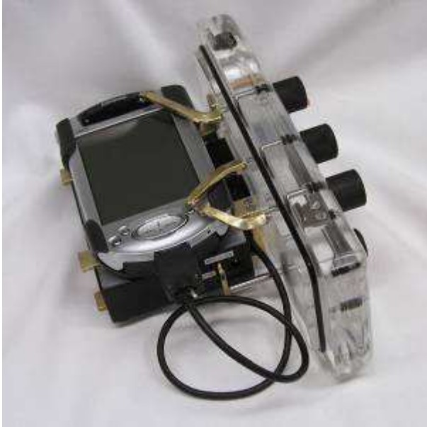
Figure 8 The spectrometer and iPAQ are fixed in brackets which are connected to the right side of the housing.
