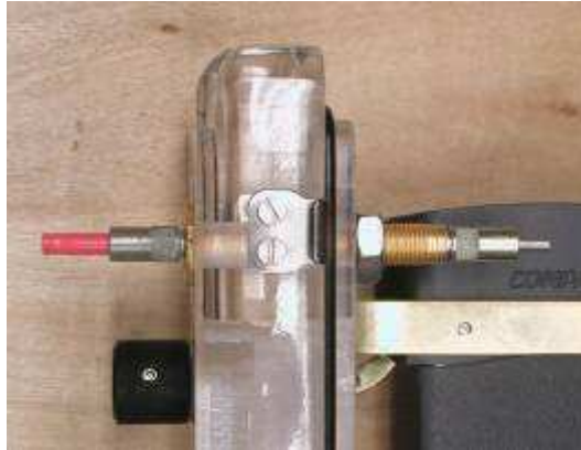
Figure 3 Vacuum feed-through for optical cable.
