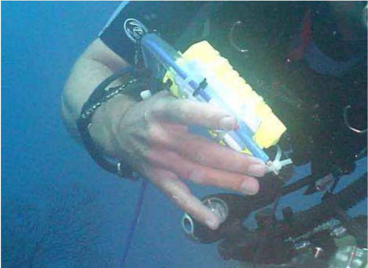
Figure 12 Dive torch attached to fibre optic cable
