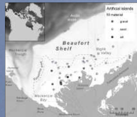
Figure 1 Location map of the Canadian Beaufort Shelf showing the distribution and fill material of artificial islands (textural dots).
