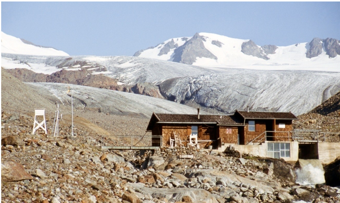
Fig.2: Hydrological part of the Vernagtbach station; from left to right: Stevenson screen and Wölfler anemometer (the same as in Fig.1), wind generator for power supply, gauging station Vernagtbach. (Photo taken by Hans Oerter, September 1979).
