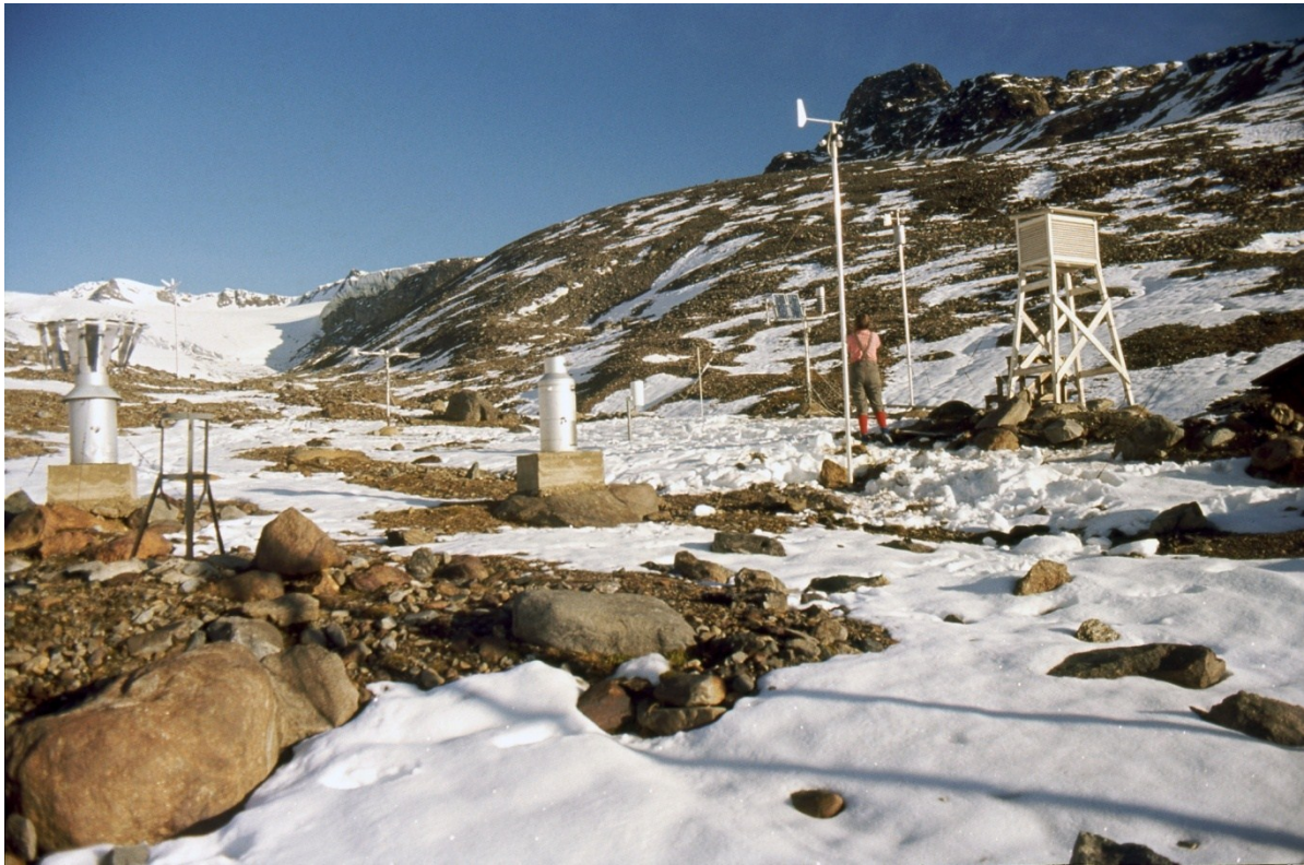
Fig. 1: Meteorological site of the Vernagtbach station; from left to right: Fuess precipitation gauge with wind shield, radiation instruments, Belfort precipitation gauge, Gertsch tipping bucket, solar panel and hair hygrometer, Thies anemometer, Wölfler anemometer, Stevenson screen with air temperature and BTW long-term thermo- and hygrograph inside. (Photo taken by Markus Weber, October 1984).
