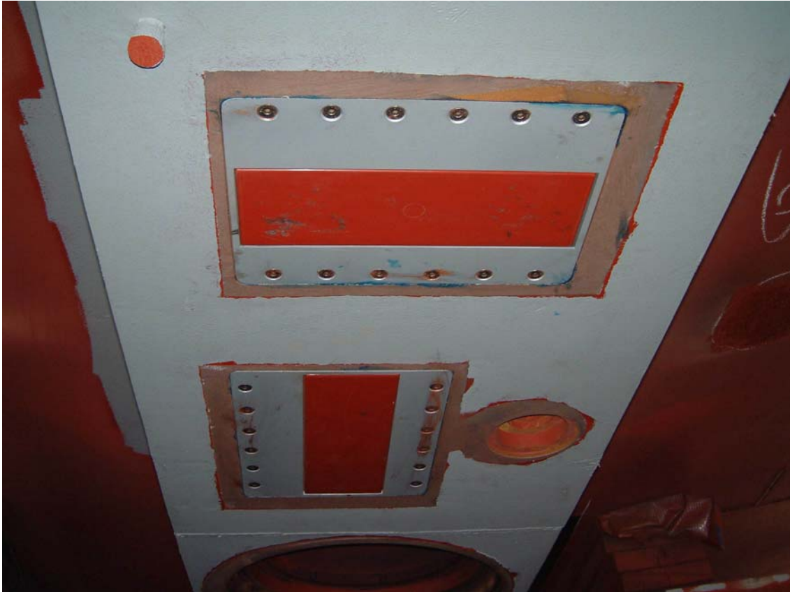
Figure 12 Installation of the 2x2 degrees transducer array on “HMS Endurance”
