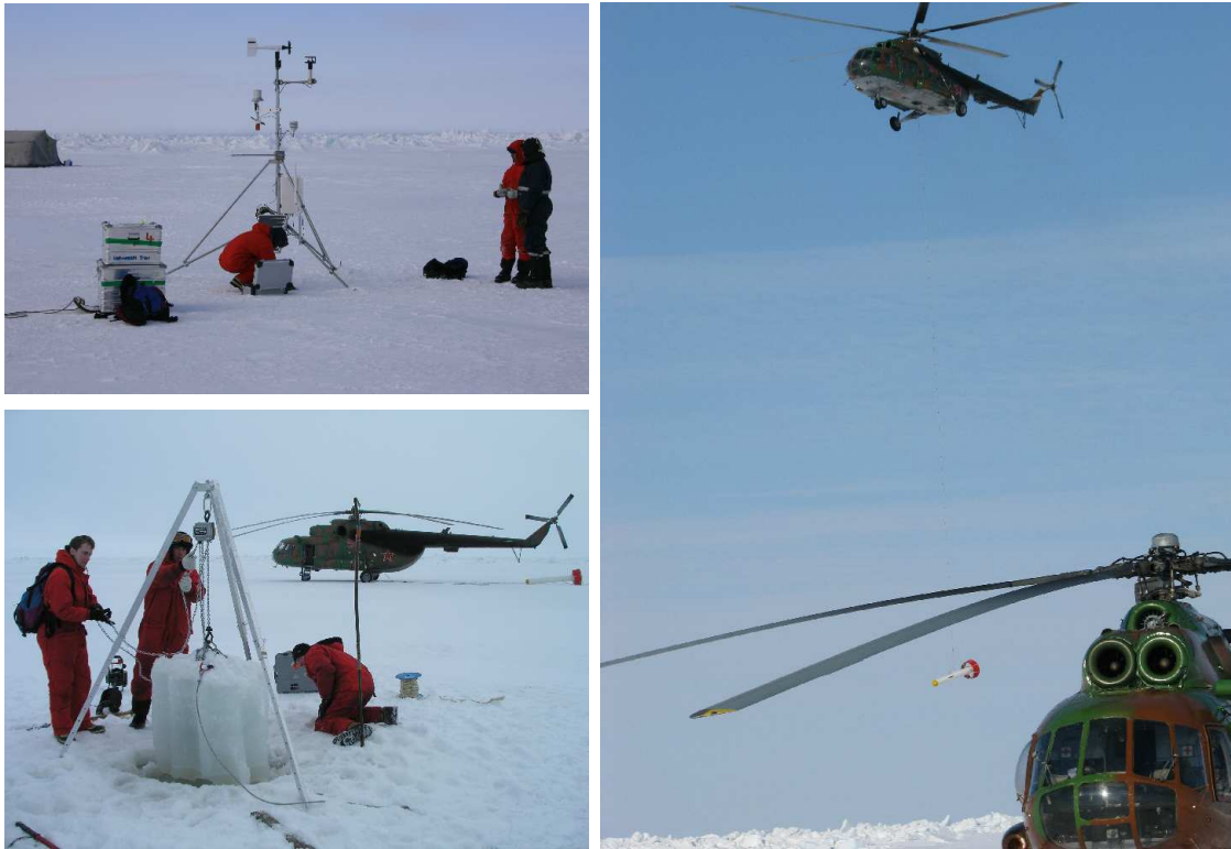
Figure 1.4: Scientific activities during TD XIII expedition. The upper left panel shows the assembling of a weather station. The lower left panel pictures the recovery of a mooring deployed for 1 month under the fast ice by means of a tripod. The right figure shows the so called EM-Bird, an airborne electromagnetic (EM) system towed by a Russian MI-8 helicopter 15 meters above the ice surface. The instrument utilises the contrast of electrical conductivity between sea water and sea ice to determine the distance to the ice-water interface (ice thickness).
