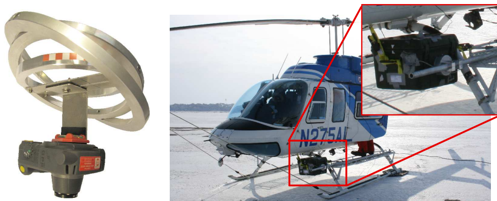
Figure 4.1: (Left) RICOH® camera 500SE placed on a two-axis gimbal for tilt compensation. (Right) Photograph of HELIOS (HELicopter-borne Ice Observation System) mounted on a BELL Helicopter.
