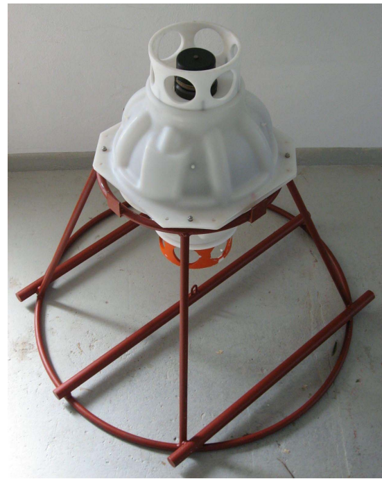
Figure 2. PACT bottom unit and steel stand. The black cylinder at the top is the HAM.NODE modem; the burn-wire release of the BU is located in the lower cage. For deployment, additional weights are attached between the release and the steel stand.
