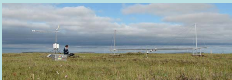
Short and longwave radiation scanner on Samoilov Island, Lena-Delta, Siberia
