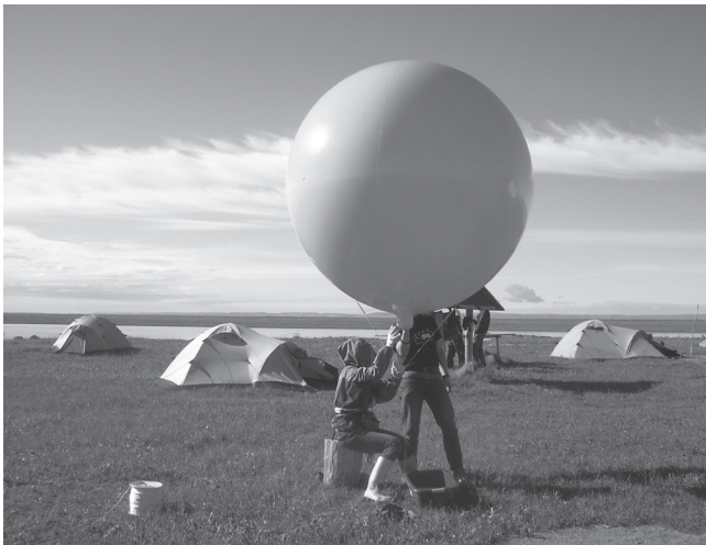
Figure 4. Tethered balloon, filled with helium, diameter 2–3 m.
