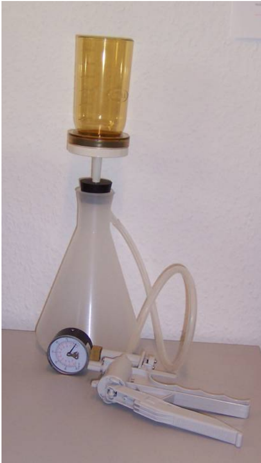
Figure 2. Filtration equipment and filtration device
