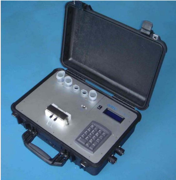
Figure 9. Semi-automated portable ALGADEC device
