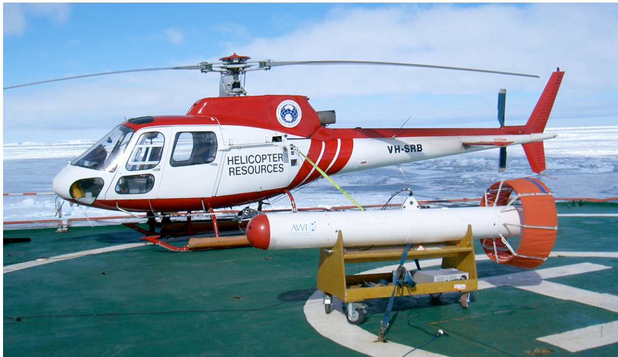
Figure 1: AWI's small sized HEM bird on RSV "Aurora Australis" in Antarctic pack ice.
