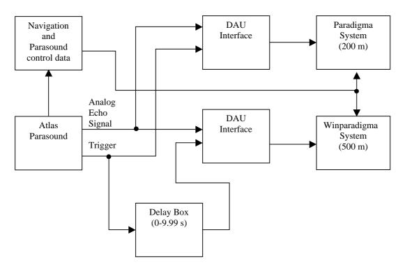
Fig. 3.1: Flare registration system of the SO178-KOMEX cruise.
