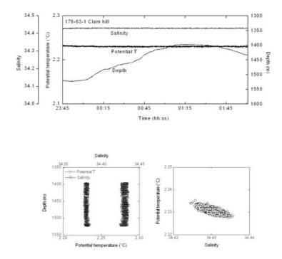
*Fig.* 8.24: Depth, salinity and potential temperature profiles obtained with the OFOS-mounted CTD during OFOS station S0178-50-1 at Clam Hill.
