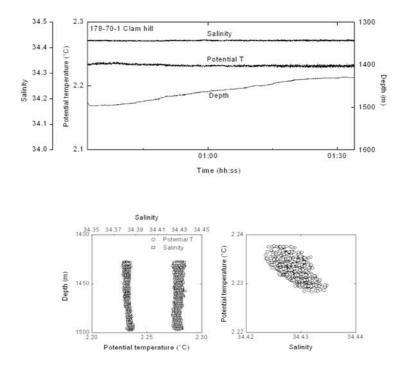
Fig. 8.26: Depth, salinity and potential temperature profiles obtained with the OFOS-mounted CTD during OFOS station S0178-70-1 at Clam Hill.
