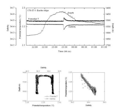
*Fig.* 8.23: Depth, salinity and potential temperature profiles obtained with the OFOS-mounted CTD during OFOS station SO178-57-1 at Barite Ridge. An anomaly in salinity and potential temperature can be seen at 23:25.
