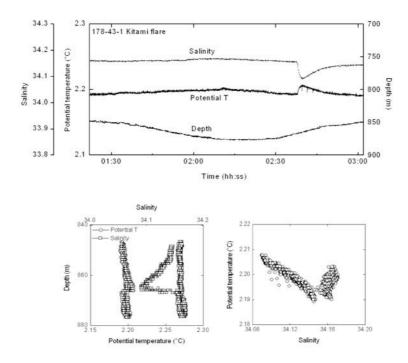
**Fig. 8.20:** Depth, salinity and potential temperature profiles obtained with the OFOS-mounted CTD during OFOS station SO178-43-1 at theKitami Flare. An anomaly in salinity and potential temperature can be seen at 02:40.
