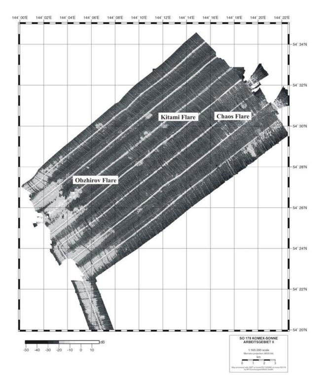
*Fig. 8.4:* General backscatter map of the Sakhalin Slope sector investigated during cruise SO178-KOMEX. The Obzhirov, Kitami and Chaos Flare areas are characterized by high backscatter.
