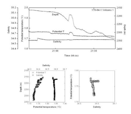
*Fig.* 8.28: Depth, salinity and potential temperature profiles obtained with the OFOS-mounted CTD during OFOS station SO178-84-1 at Volcano No. 1. The anomaly between 21:10 and 21:14 was produced by hauling the OFOS due to technical problems with the video equipment.
