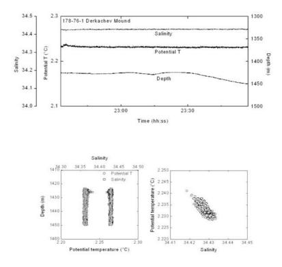
Fig. 8.27: Depth, salinity and potential temperature profiles obtained with the OFOS-mounted CTD during OFOS station S0178-76-1 at the Derkachev Mound.
