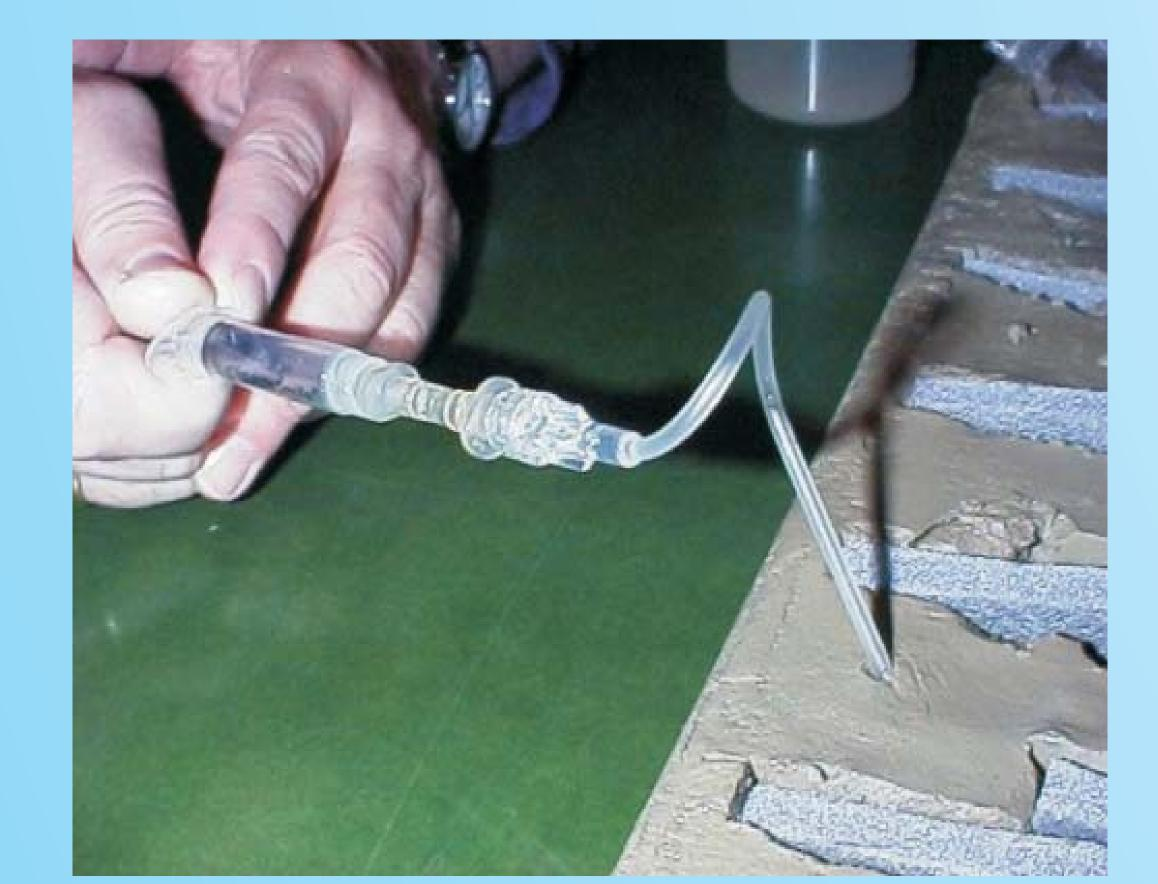
Fig. 2: Rhizon pore water sampling in marine sediment cores, to our knowledge the first attempt to collect pore water samples from marine sediments using rhizon soil moisture samplers..
