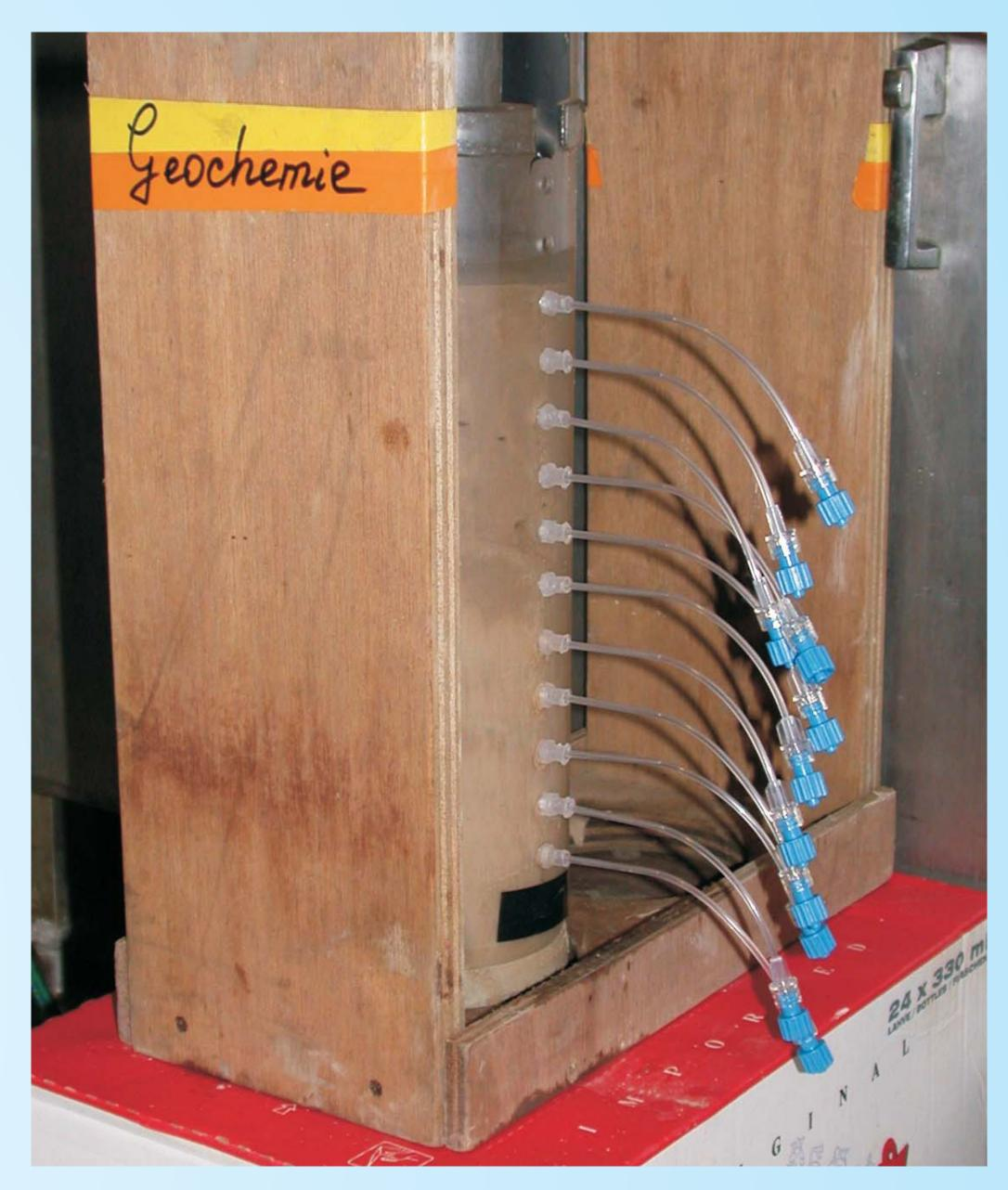
Fig. 8: **Porewater sampling from MUCs.** Multicorer liner tube on a Polarstern Cruise with rhizons installed through predrilled holes in the liner wall. Sampler connectors are sealed by blue caps until syringes are attached. Vertical distance of sampling points is 2 cm.
