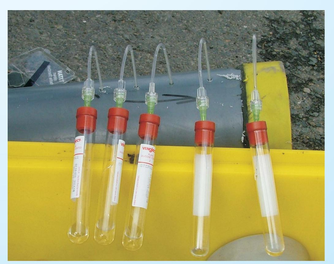
Fig. 7: Pore water sampling from a core liner using Rhizon samplers attached to a needle and blank vacutubes. For special purposes also preloaded vacutubes may be used
