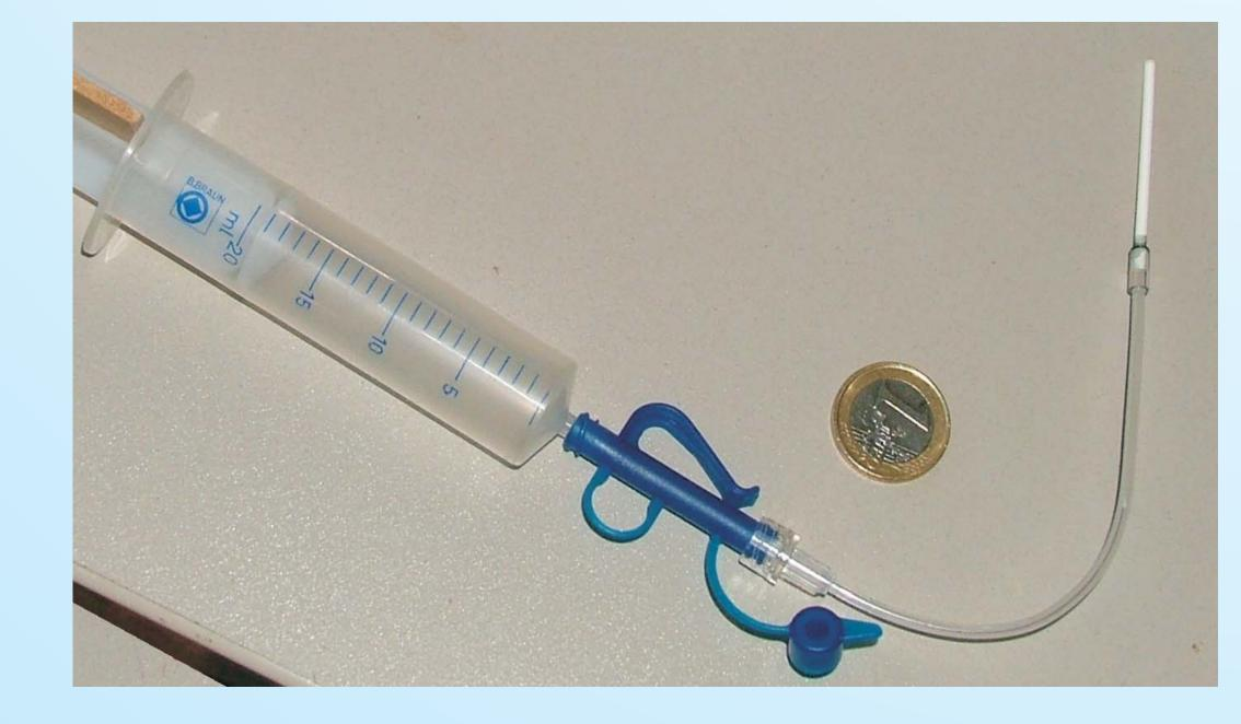
Fig. 5: **Rhizon Core Solution Sampler** connected to a 20 mL disposable syringe. Vacuum is simply applied by pulling the plunger and keeping it in place with a spacer.
