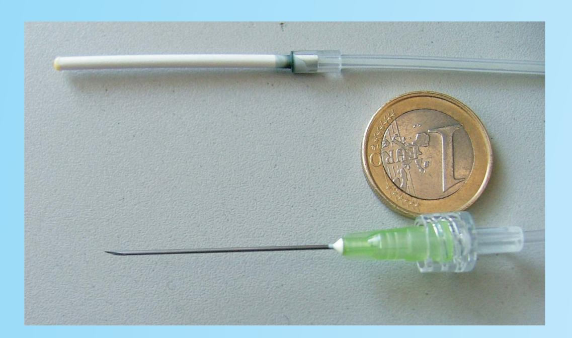
Fig. 1: **Rhizon Core Solution Sampler**, 50mm length, 2.5mm diameter (Rhizosphere Research Products, Wageningen NL). The hydrophilic microporous tube (white) is supported by a nylon wire. The sampler is connected to Tygon tubing.
