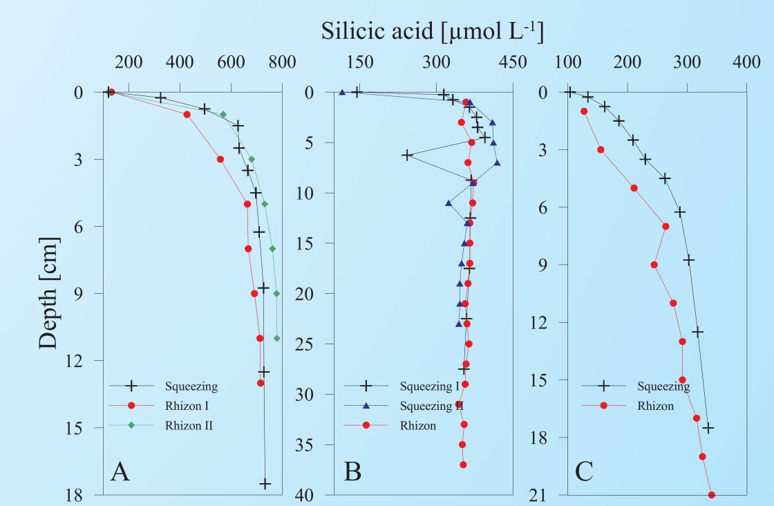
Fig. 9: Comparison between rhizon sampling and conventional squeezing. Porewater concentrations of silicic acid in the MUC tube above measured from both rhizon sampling and conventional sampling by pressure filtration of the sediments.
