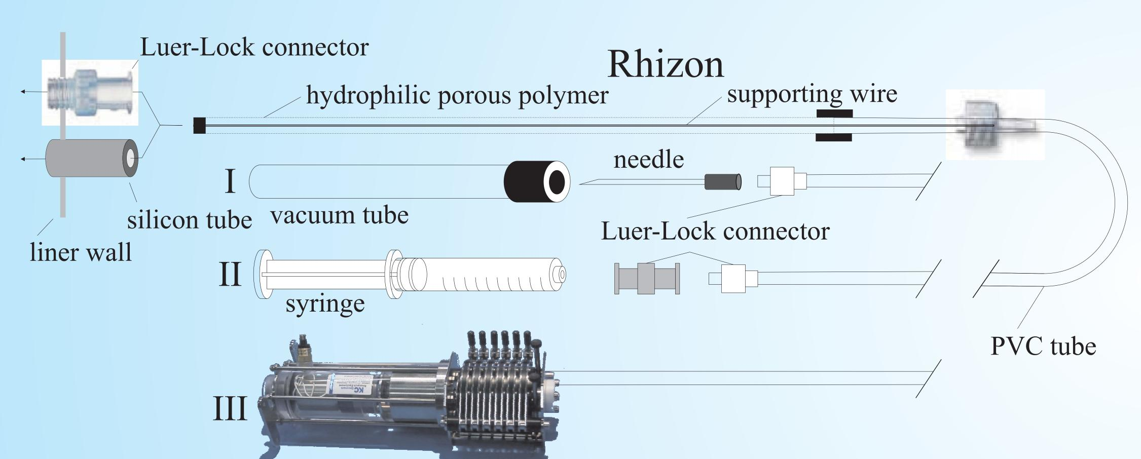
Fig. 3: **Rhizon sampling**: Vacuum may be applied by either I a needle inserted into a blank vacutube, II a syringe with the plunger kept open by a spacer or III by a peristaltic pump. The peristaltic pump shown (KC Denmark deep sea peristaltic pump) is suitable for underwater use.
