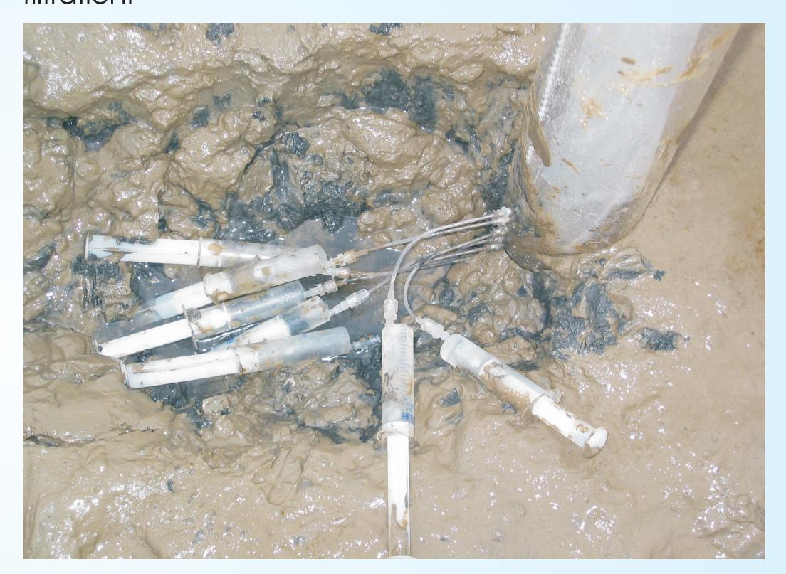
Fig. 6: **Manual semi In situ sampling**. A liner driven is into wadden sediments then one wall is cleared and rhizon samplers are pushed through predrilled holes in the wall. Sampling by disposable syringes with spacer. Despite all the "dirt" on the picture the samples are clean and 0.15micron filtrated
