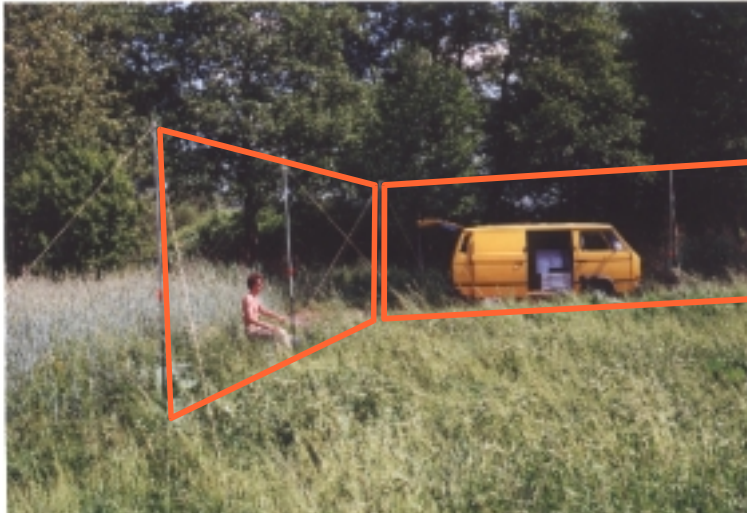
Figure 3-7 Built up transmitter loops in the field. The loop cables are highlighted by orange lines.
