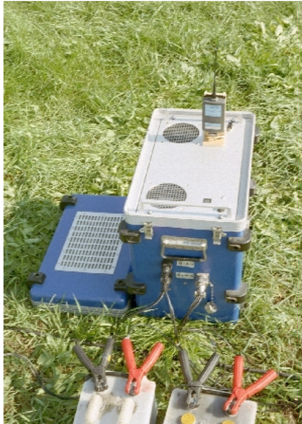
Figure 3-10 The reworked transmitter system with radio modem.
